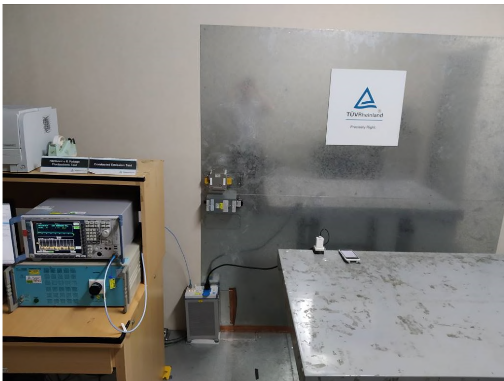
Photograph 6: Set-up for for AC Mains (Front)
