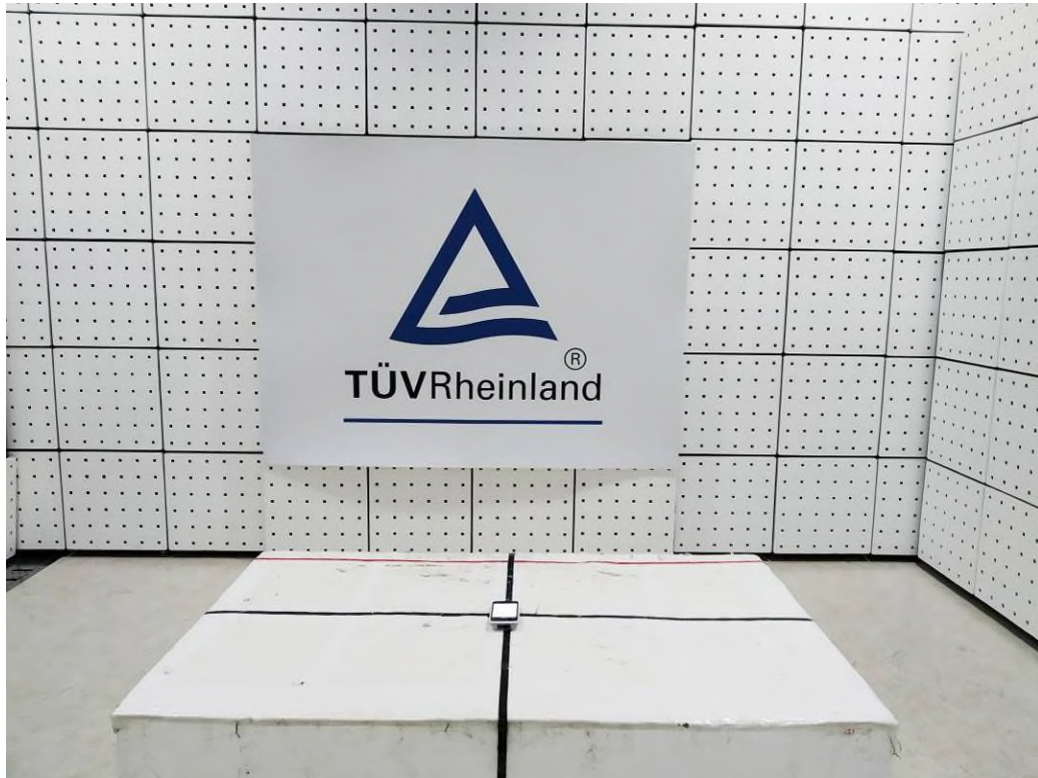
Photograph 2: Set-up for Spurious Emissions (Back View 1)
