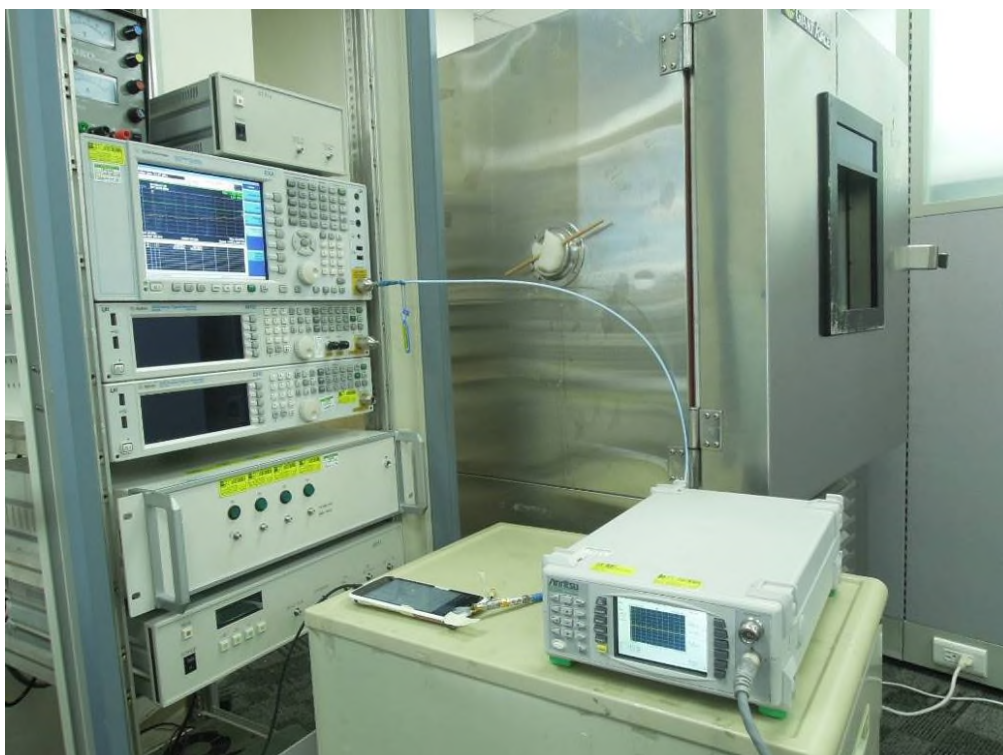
Photograph 4: Set-up for Conducted testing
