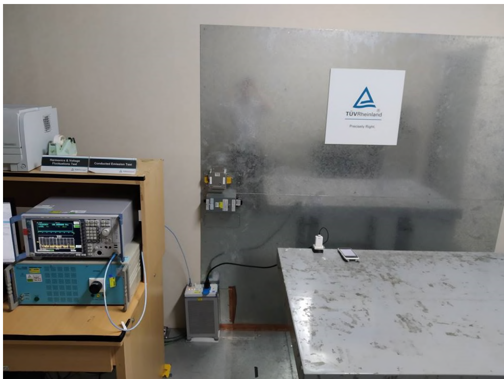
Photograph 5: Set-up for for AC Mains (Front)
