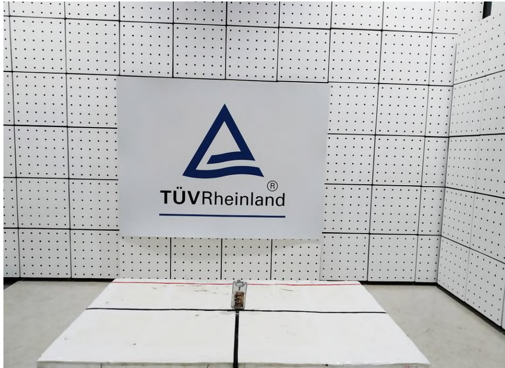
Photograph 2: Set-up for Radiated Emissions RX (Front View)
