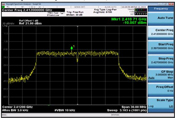
**Power Spectral Density Test Plot (CH-Mid)**
