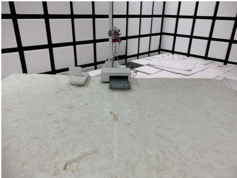
Radiated spurious emission Test Setup-2(Above 1GHz)
