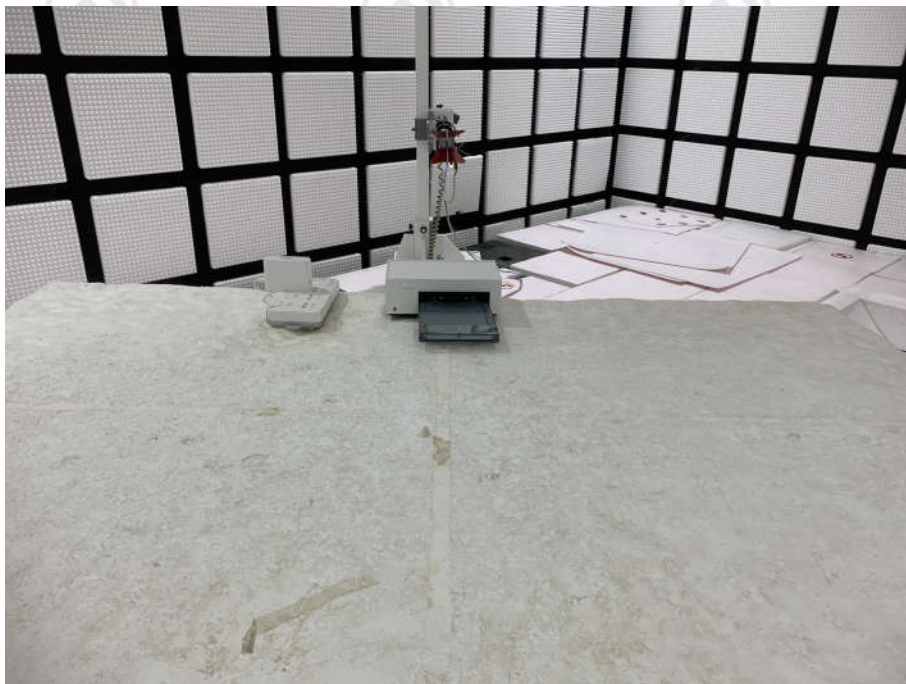
Radiated spurious emission Test Setup-2(Above 1GHz)
