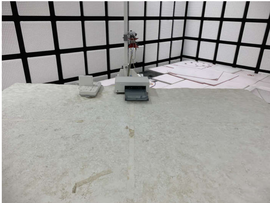
Radiated spurious emission Test Setup-2(Above 1GHz)
