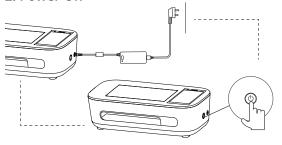
Connect the power cord to the adapter and socket. To ensure the normal operation of the device, please use 100-240 volts AC power. Connect the adapter to the power interface of the device; Install the blade kit on the clamp to ensure it is fixed correctly. After connecting, press [PowerSwitch] to start the device.
