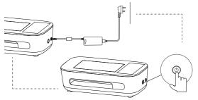
Connect the power cord to the adapter and socket. To ensure the normal operation of the device, please use 100-240vdts AC power. Connect the adapter to the power interface of the device; Install the blade kit on the clamp to ensure it is fixed correctly. After connecting, press [PowerSwitch]to start the device.
