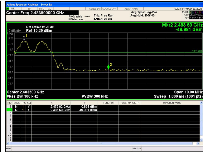
Out Of Band Emission(Right) GFSK_DH5_Channel Hopping
