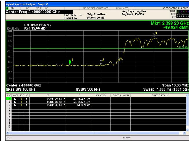
Out Of Band Emission(Left) 8DPSK_3-DH5_Channel Hopping
