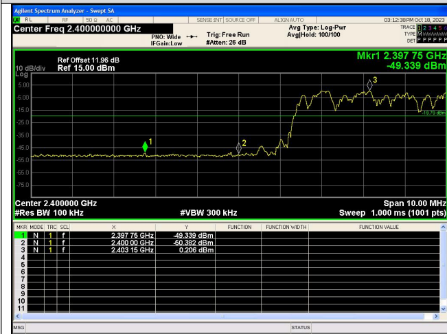
Out Of Band Emission(Left) 8DPSK_3-DH5_Channel Hopping
