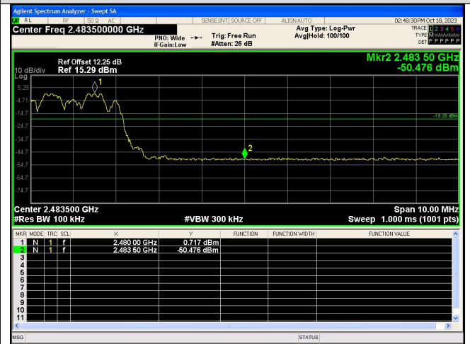
Out Of Band Emission(Right) \pi/4 DQPSK_2-DH5_Channel Hopping
