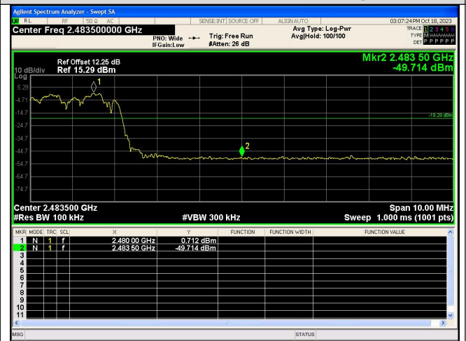
Out Of Band Emission(Right) 8DPSK_3-DH5_Channel Hopping
