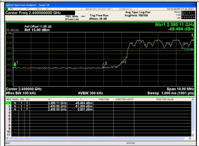
Out Of Band Emission(Left) \pi/4 DQPSK_2-DH5_Channel Hopping
