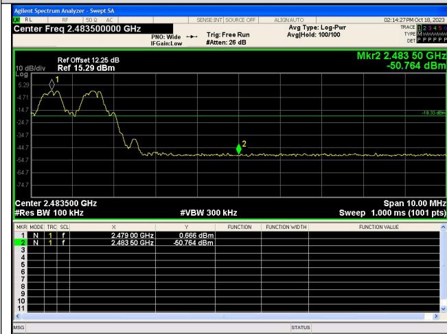
Out Of Band Emission(Right) GFSK_DH5_Channel Hopping
