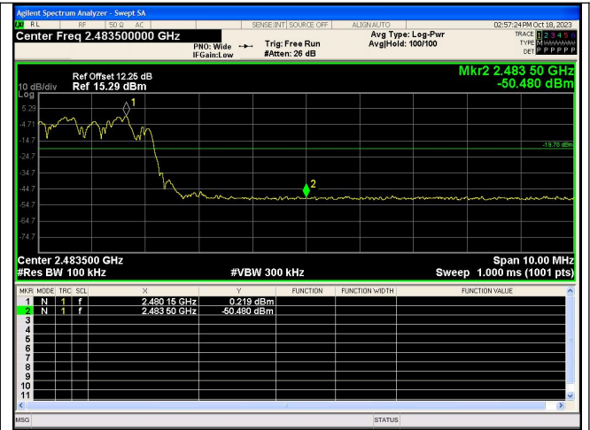
Out Of Band Emission(Right) 8DPSK_3-DH5_Channel Hopping
