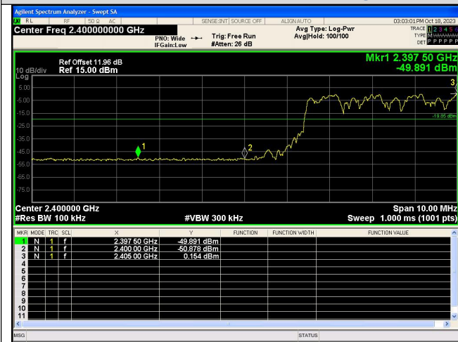
Out Of Band Emission(Left) 8DPSK_3-DH5_Channel Hopping
