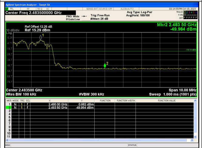
Out Of Band Emission(Right) 8DPSK_3-DH5_Channel Hopping
