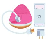
You may charge using any USB outlet, a wall socket mobile phone charger or even a laptop. The LEDs would blink when the battery is charging and stay steady once charged.
