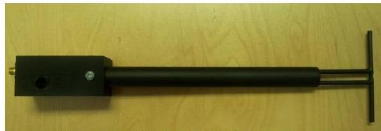
Figure 1 – MVG COMOSAR Validation Dipole
