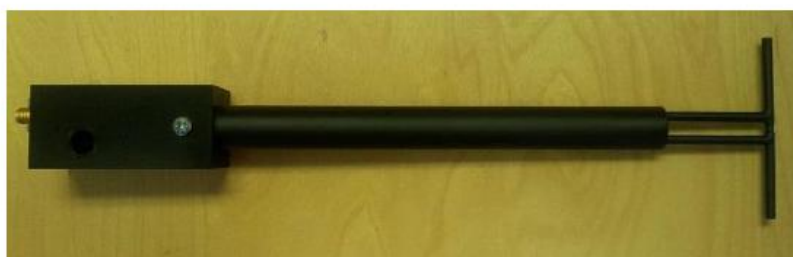
Figure 1 – MVG COMOSAR Validation Dipole
