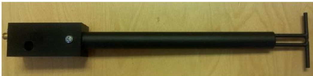
Figure 1 – MVG COMOSAR Validation Dipole
