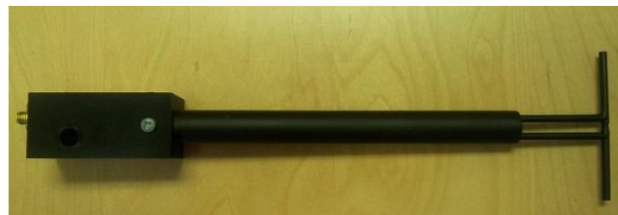
Figure 1 – MVG COMOSAR Validation Dipole
