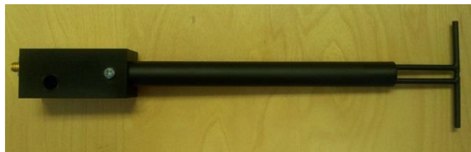
Figure 1 – MVG COMOSAR Validation Dipole
