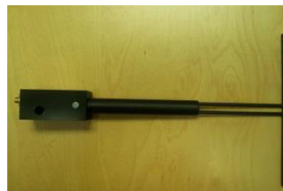
Figure 1 – MVG COMOSAR Validation Dipole
