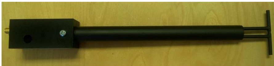
Figure 1 – MVG COMOSAR Validation Dipole
