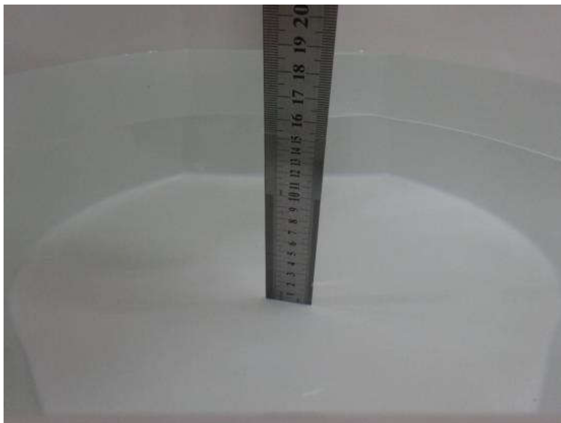
Photograph of the depth in the Head Phantom (2450MHz, 15.3cm depth)
