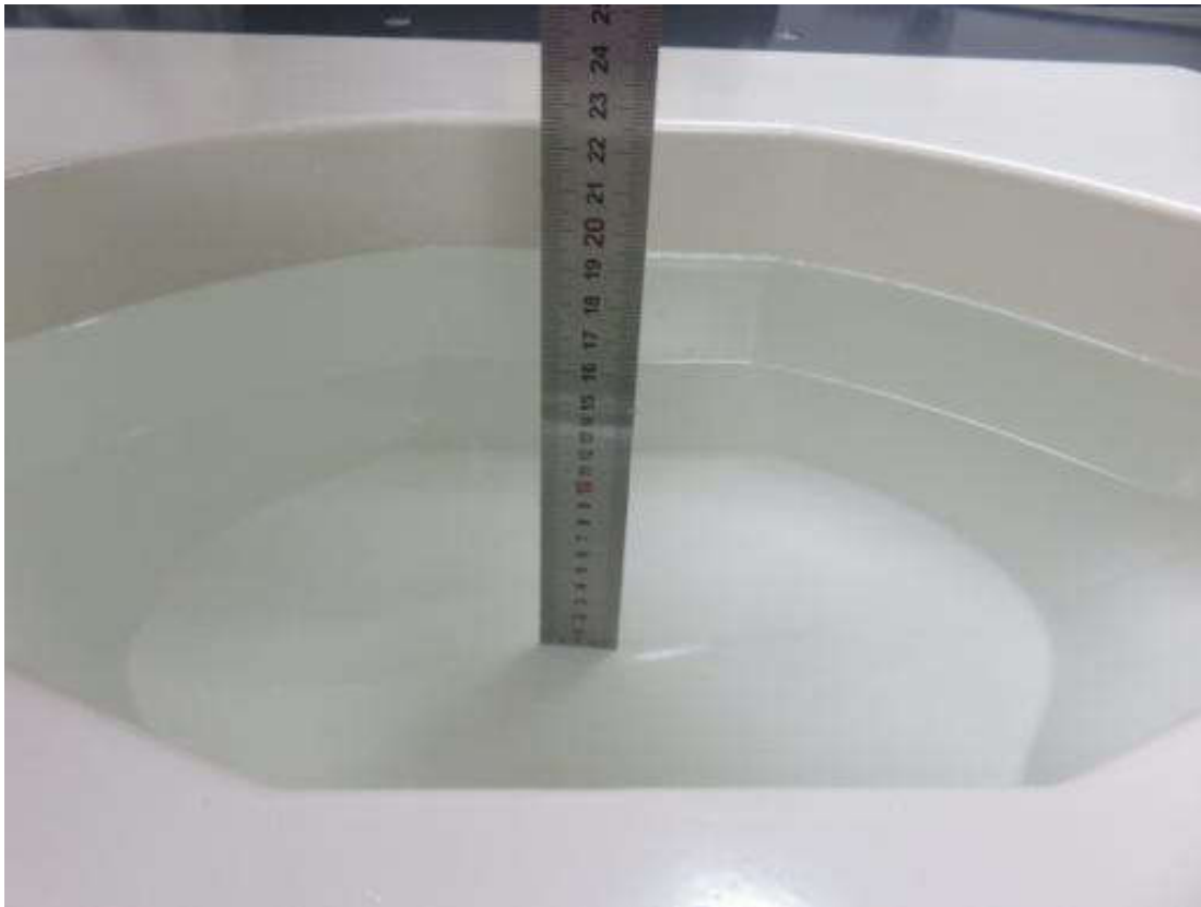
Photograph of the depth in the Body Phantom (5-6GHz, 15.2cm depth)
