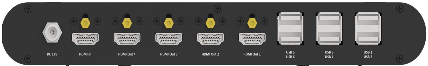
Figure 2 Interface definition diagram-4HDMI
