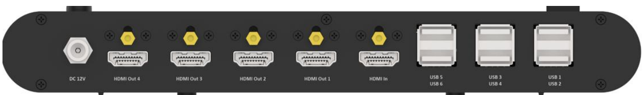
Figure 2 Interface definition diagram-4HDMI
