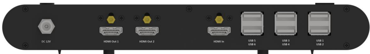
Figure 3 Interface definition diagram-2HDMI
