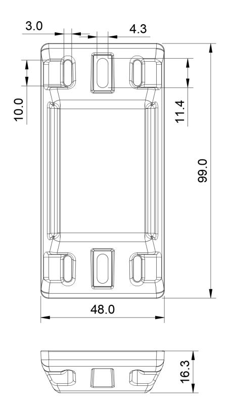
All dimensions are in millimeters (mm).
