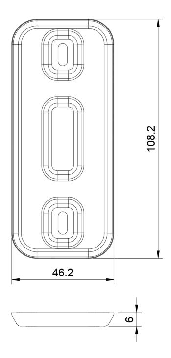
All dimensions are in millimeters (mm).
