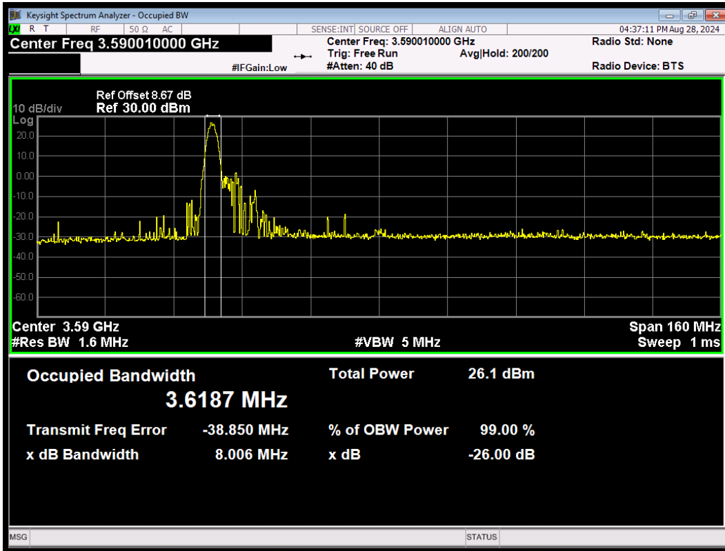
MIMO\PC3\NR n48 SCS=30kHz CP_64QAM BW=80MHz Channel=639334 RB=1@0
