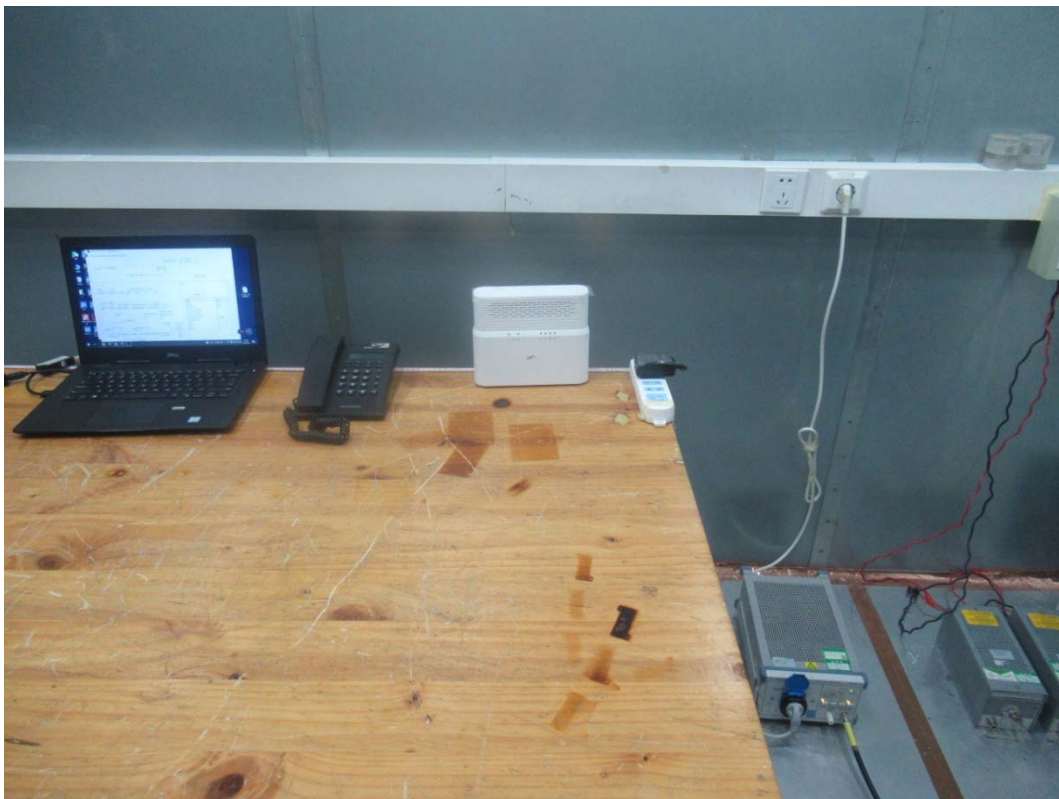
Picture 2 Conducted Emission Test Setup
