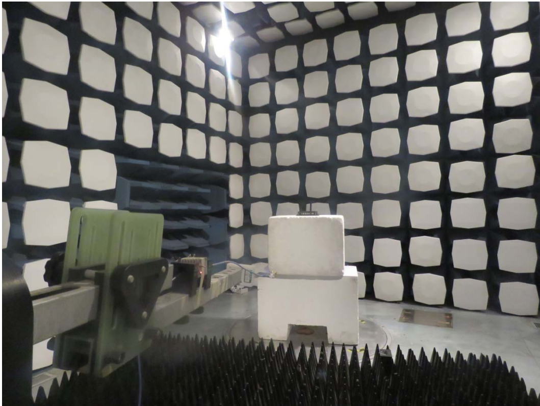
Picture 1 Radiated Emission Test Setup
