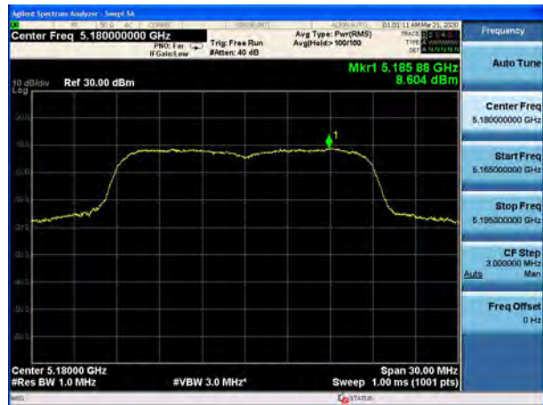
U-NII-1, 802.11ac VHT20, Channel No.: 40
