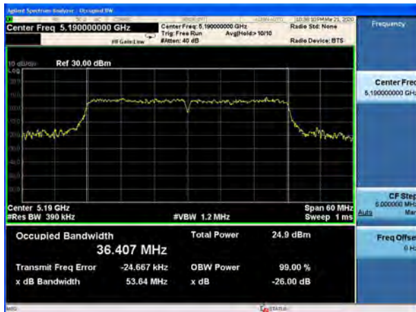
U-NII-1, 802.11n HT40 Carrier frequency (MHz): 5230
