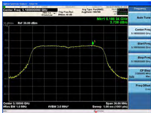
U-NII-1, 802.11ac VHT20, Channel No.: 40
