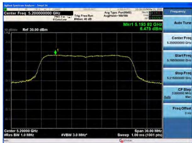
U-NII-1, 802.11ac VHT20, Channel No.: 48
