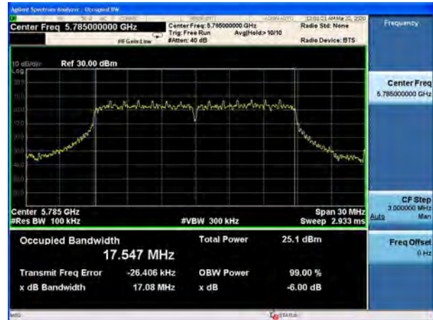
U-NII-3, 802.11n HT20 Carrier frequency (MHz): 5825
