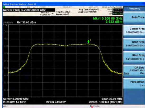
U-NII-1, 802.11ac VHT20, Channel No.: 48
