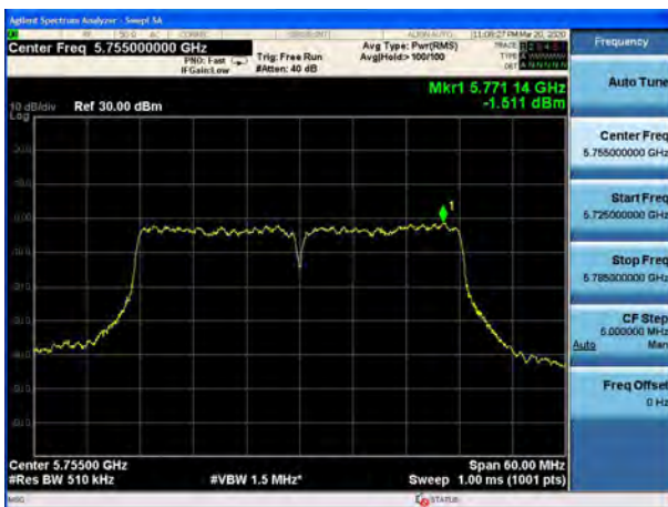
U-NII-3, 802.11ac VHT40, Channel No.: 151
