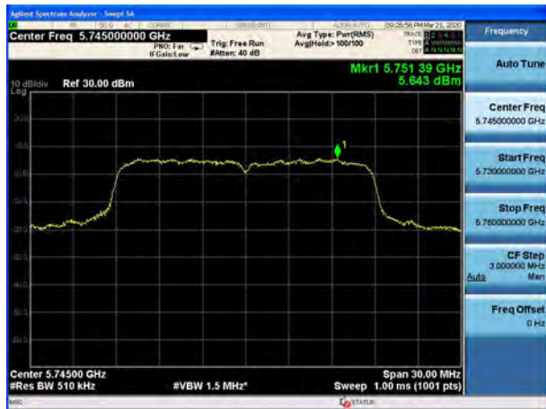
U-NII-3, 802.11ac VHT20, Channel No.: 157
