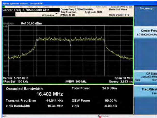
U-NII-3, 802.11a Carrier frequency (MHz): 5825
