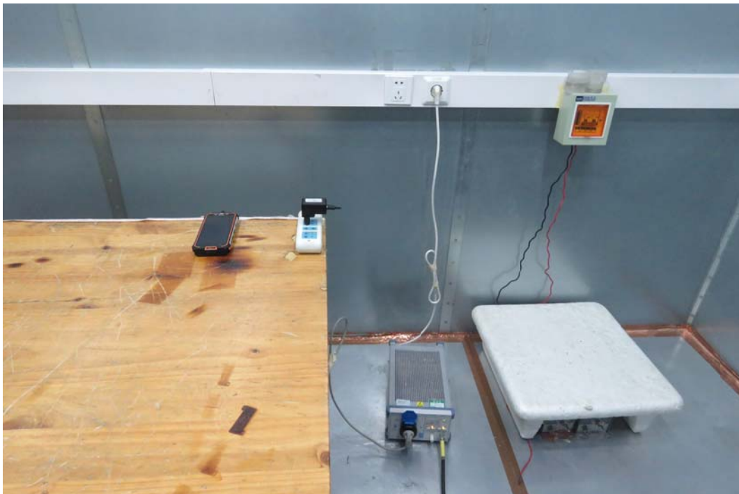
Picture 2 Conducted Emission Test Setup
