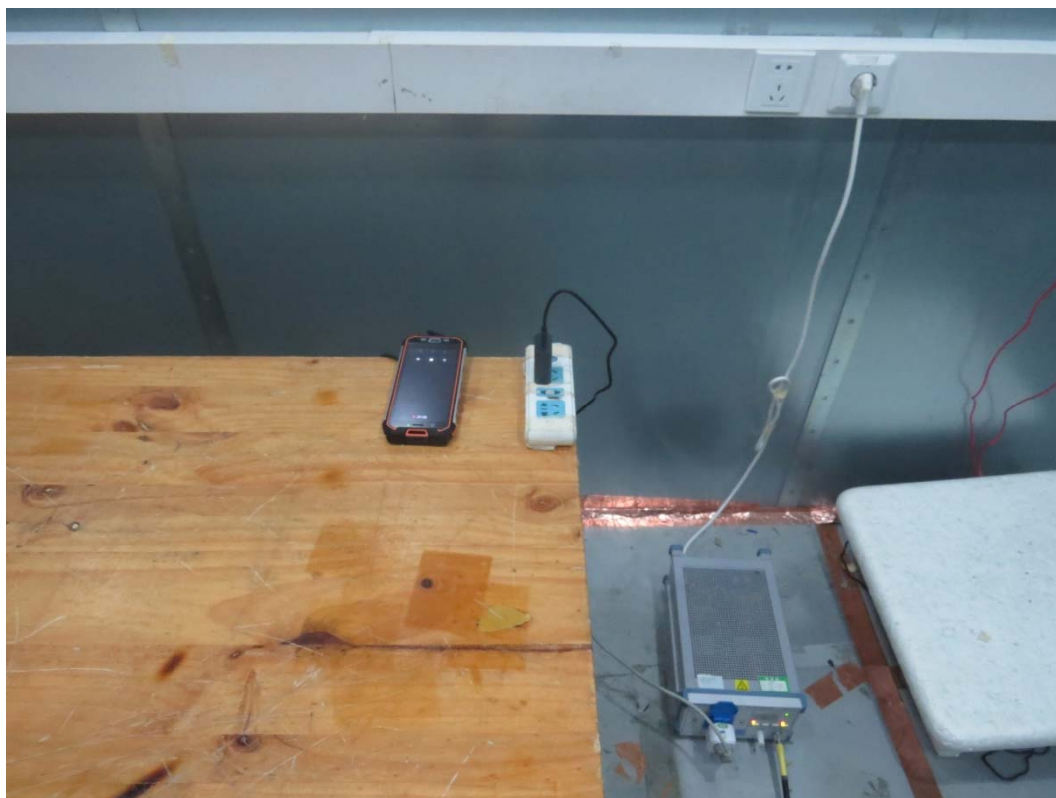
Picture 2 Conducted Emission Test Setup
