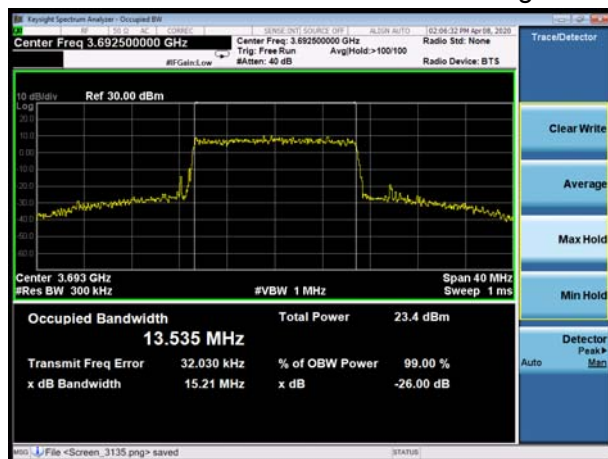
LTE Band 48 15MHz 16QAM CH-High
