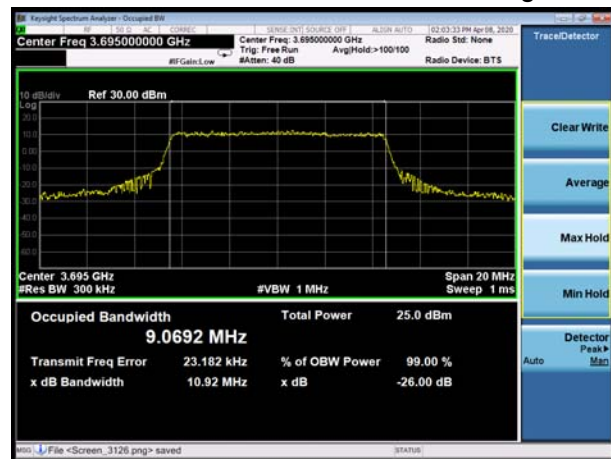
LTE Band 48 10MHz 16QAM CH-High
