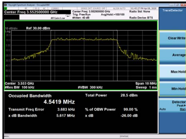
LTE Band 48 5MHz QPSK CH-Middle
