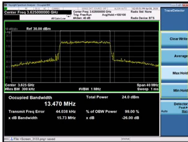
LTE Band 48 15MHz 64QAM CH-High
