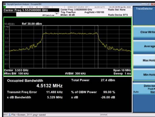
LTE Band 48 5MHz 16QAM CH-Middle
