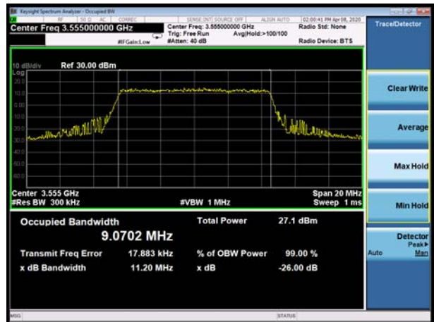
LTE Band 48 10MHz QPSK CH-Middle
