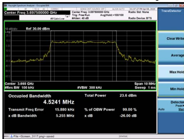
LTE Band 48 5MHz 16QAM CH-High
