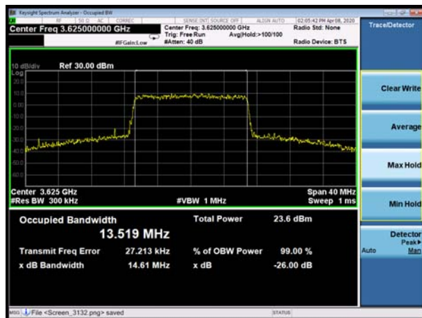
LTE Band 48 15MHz 16QAM CH-High
