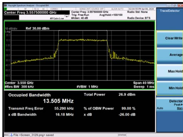
LTE Band 48 15MHz 16QAM CH-Middle
