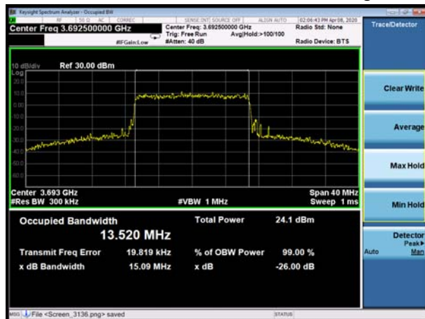
LTE Band 48 15MHz 64QAM CH-High
