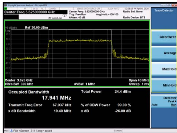
LTE Band 48 20MHz 16QAM CH-High
