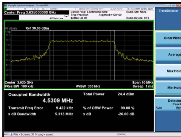
LTE Band 48 5MHz 16QAM CH-High
