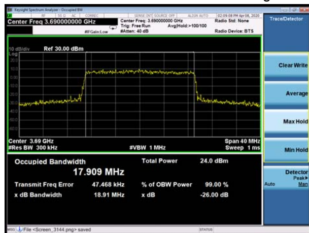
LTE Band 48 20MHz 16QAM CH-High
