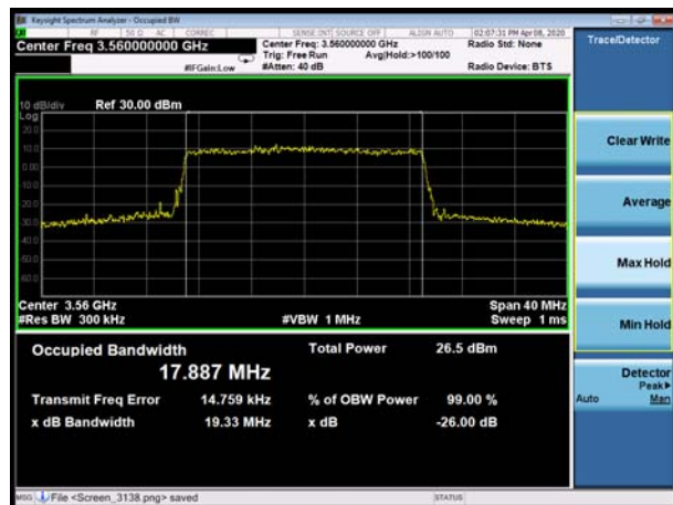
LTE Band 48 20MHz 16QAM CH-Middle
