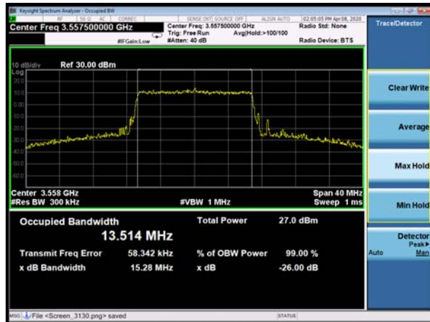
LTE Band 48 15MHz 64QAM CH-Middle
