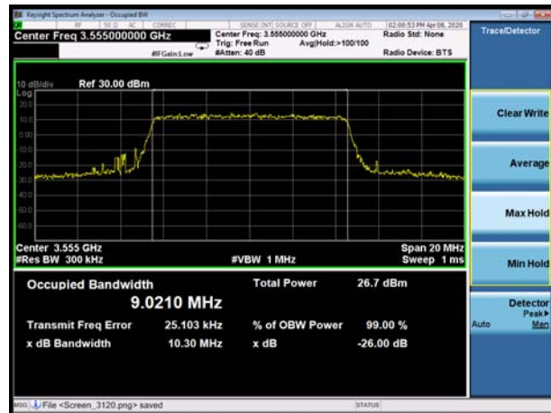
LTE Band 48 10MHz 16QAM CH-Middle
