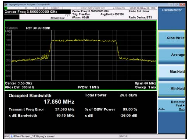
LTE Band 48 20MHz 64QAM CH-Middle
