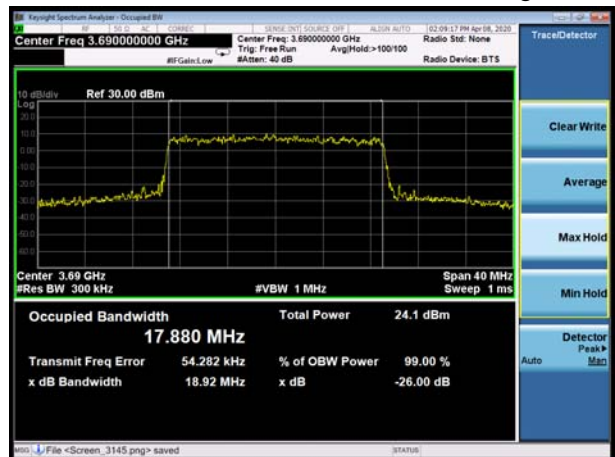
LTE Band 48 20MHz 64QAM CH-High
