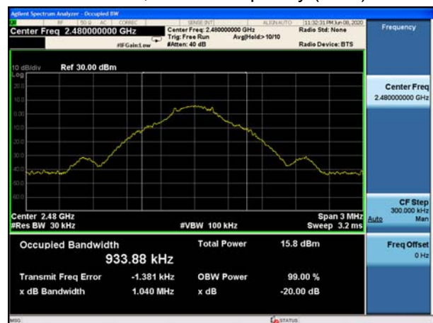
BT DH5 CH78, Carrier frequency (MHz): 2480
