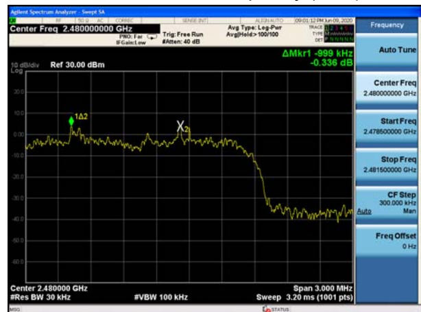
BT 2DH5 CH78, Carrier frequency (MHz): 2480
