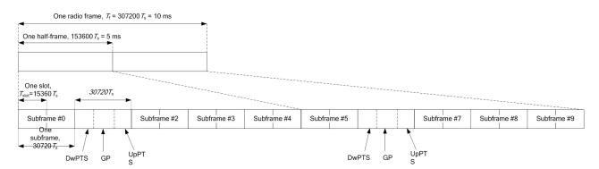
The period of the GAP is configured by base station from 66.7us to 667us, see bellows chart: 'GP' is the GAP, and one symbols is 66.7us.
