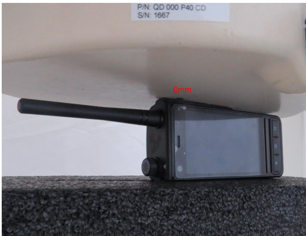
Picture 4: Right Side, the distance from handset to the bottom of the Phantom is 0mm
