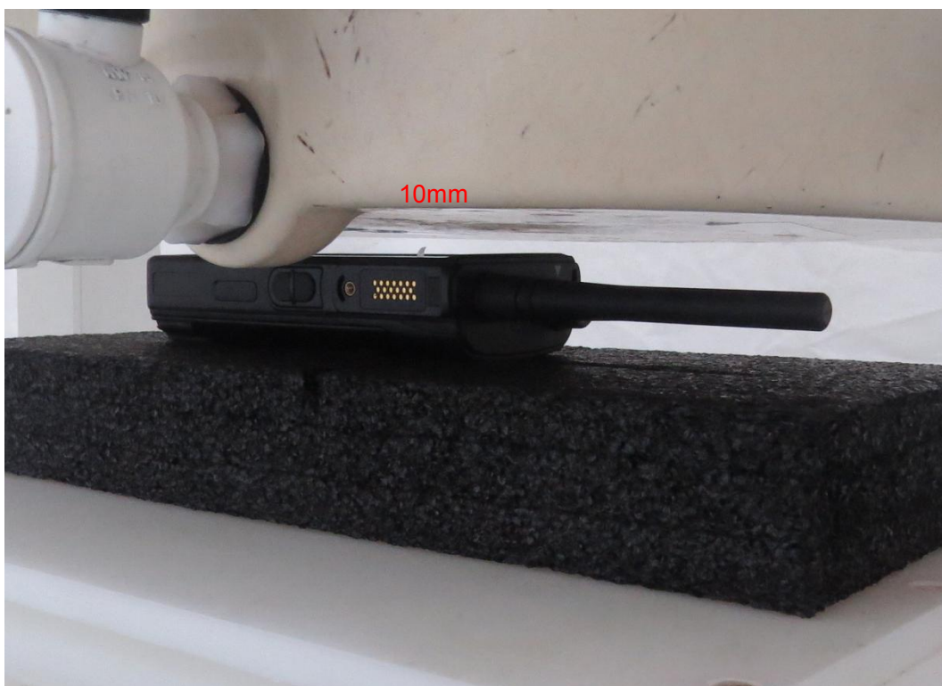
Picture 2: Front Side, the distance from handset to the bottom of the Phantom is 10mm (face up)
