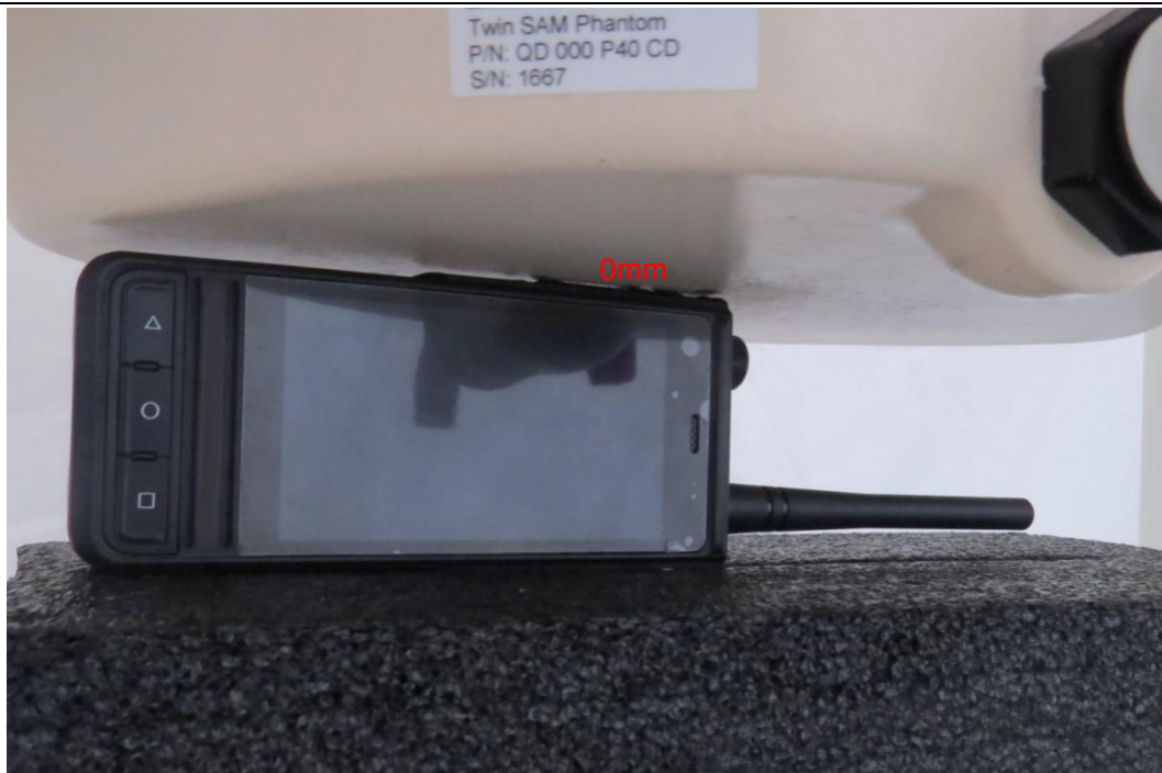
Picture 3: Left Side, the distance from handset to the bottom of the Phantom is 0mm
