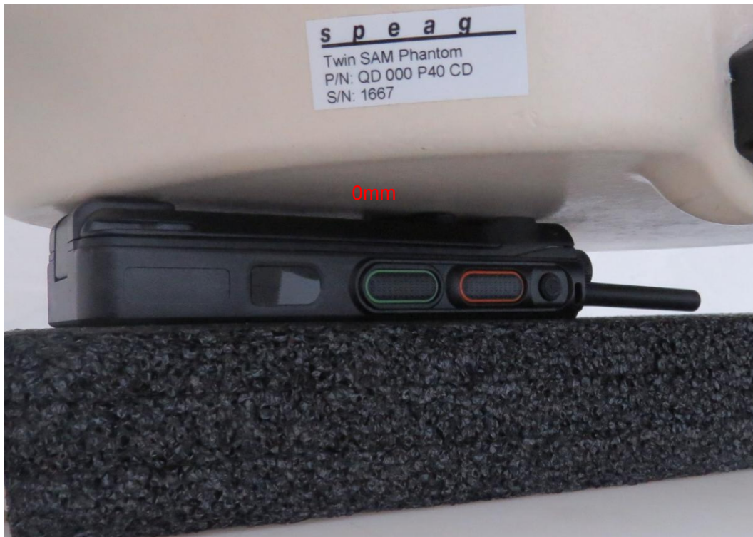
Picture 1: Back Side, the distance from handset to the bottom of the Phantom is 0mm
