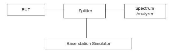
The loss between RF output port of the EUT and the input port of the tester has been taken into consideration.
