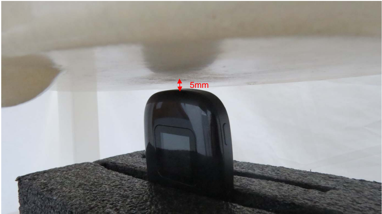
Picture 5: Top Side, the distance from handset to the bottom of the Phantom is 5mm
