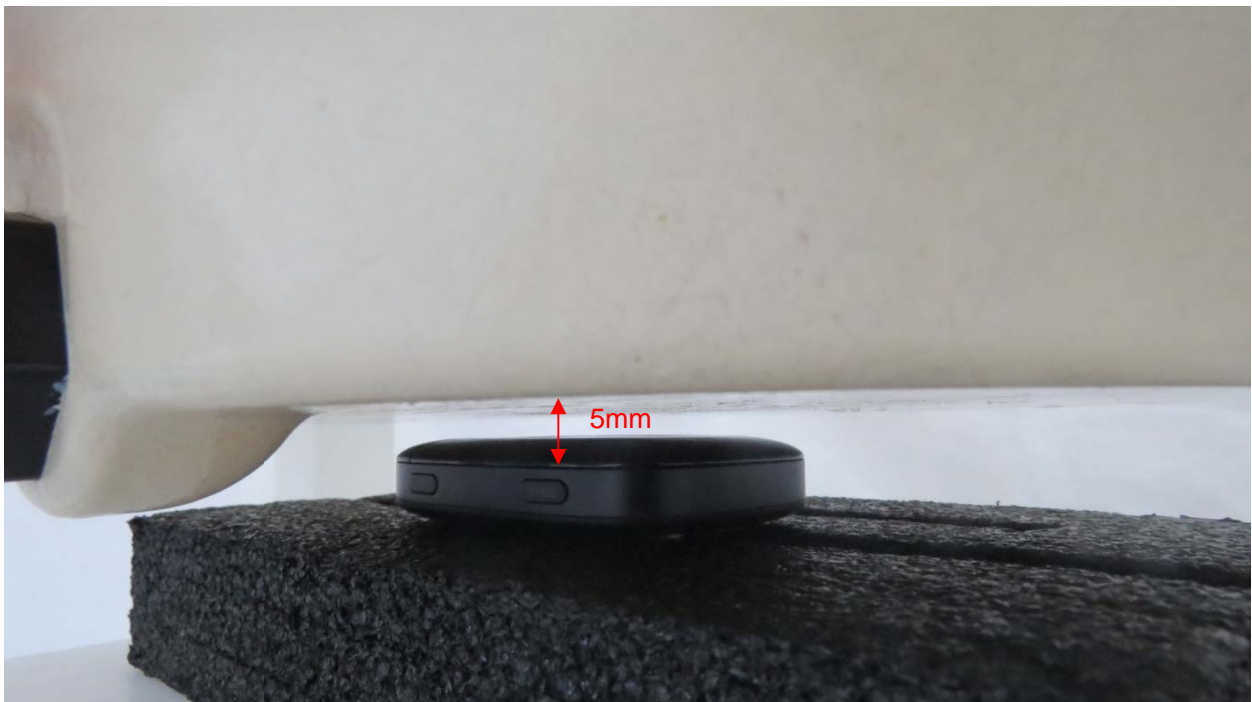
Picture 2: Front Side, the distance from handset to the bottom of the Phantom is 5mm
