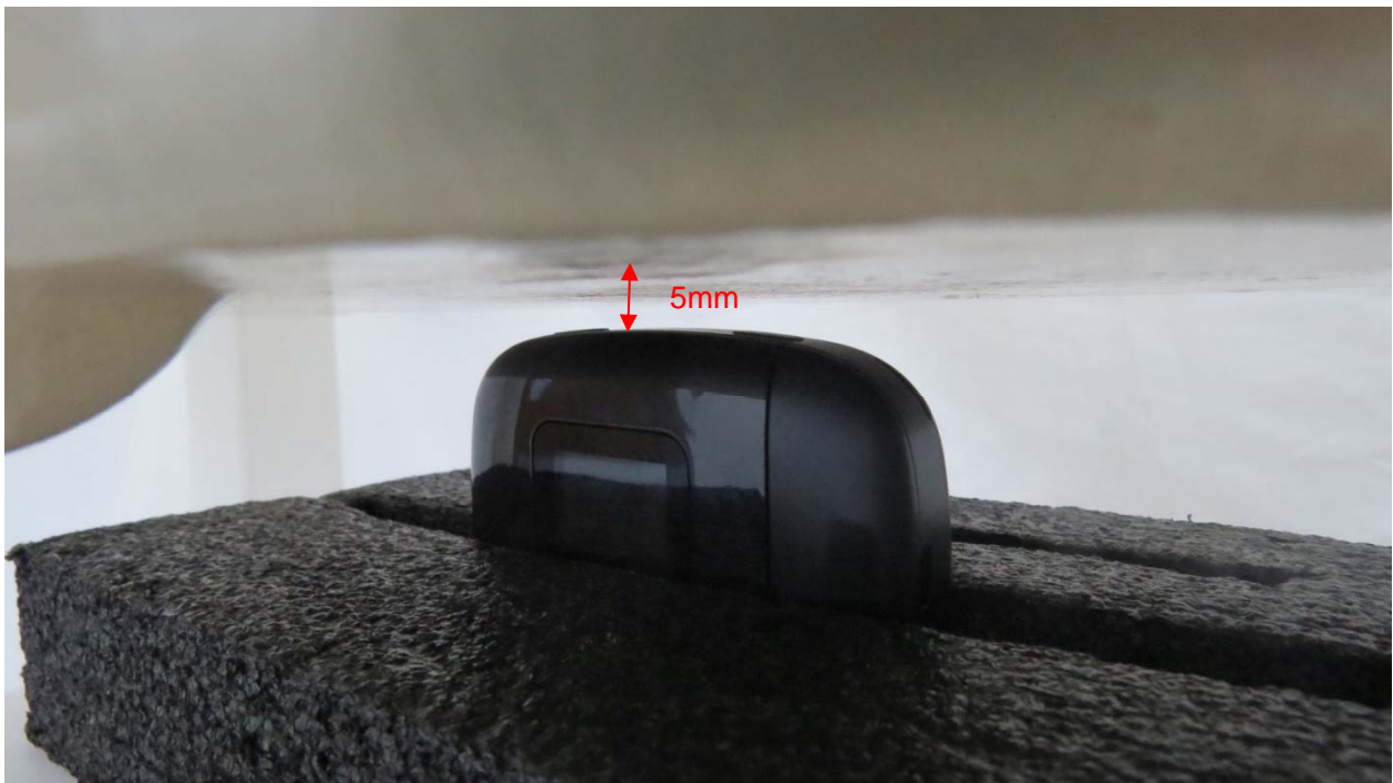
Picture 4: Right Side, the distance from handset to the bottom of the Phantom is 5mm
