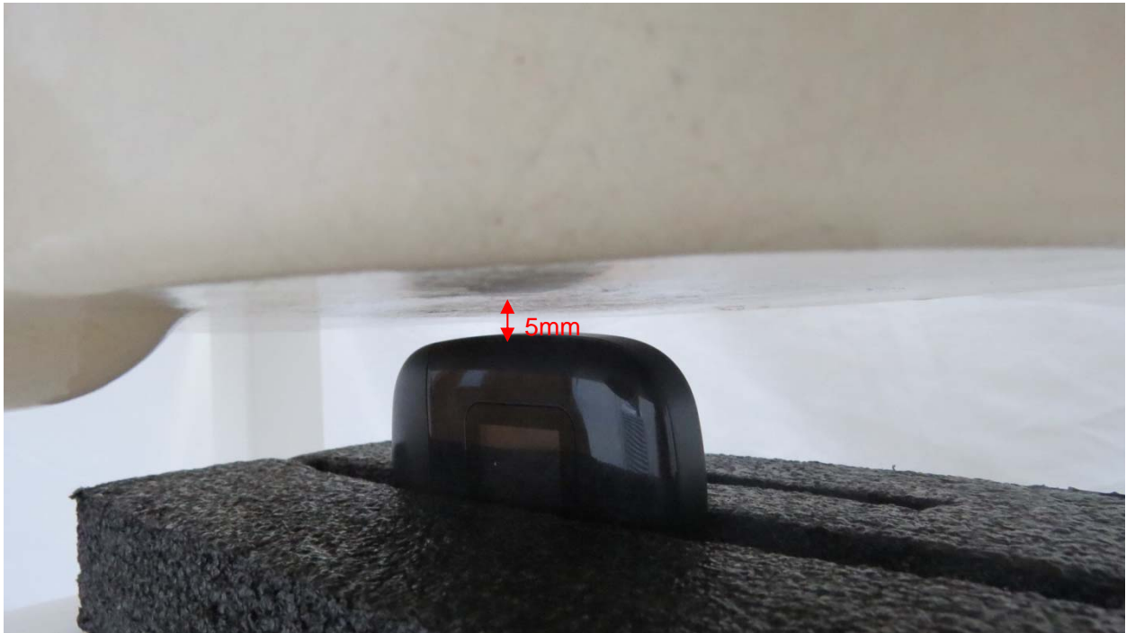
Picture 3: Left Side, the distance from handset to the bottom of the Phantom is 5mm
