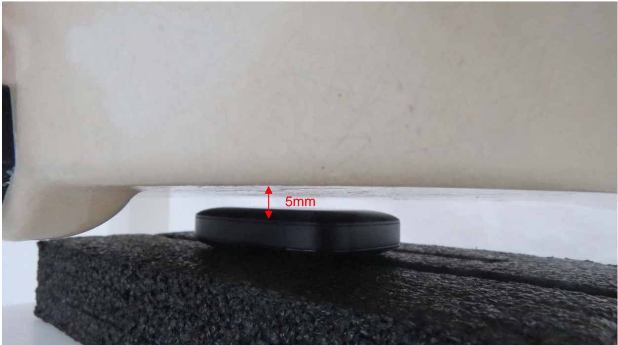
Picture 1: Back Side, the distance from handset to the bottom of the Phantom is 5mm
