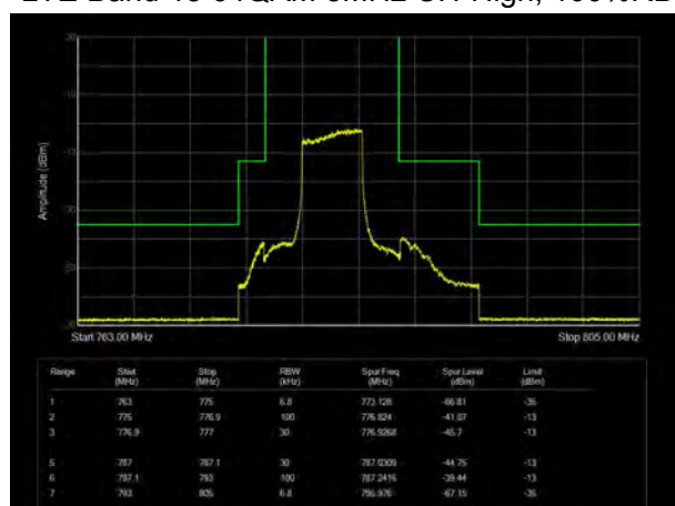
LTE Band 13 64QAM 10MHz CH-Middle, 100%RB
