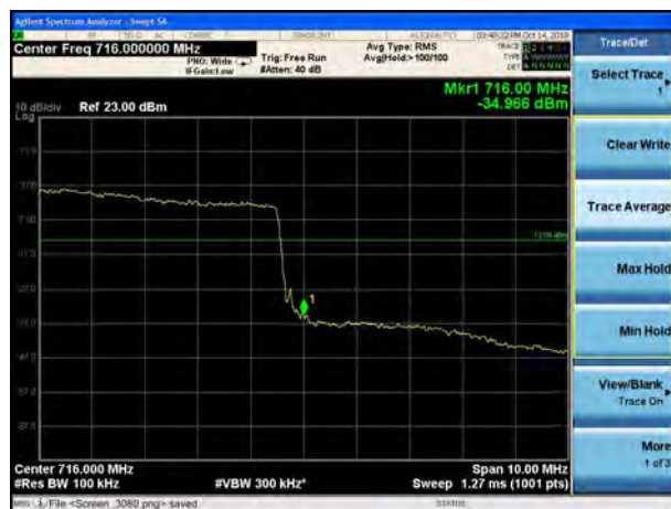
LTE Band 12 64QAM 1.4MHz CH-High, 1 RB
