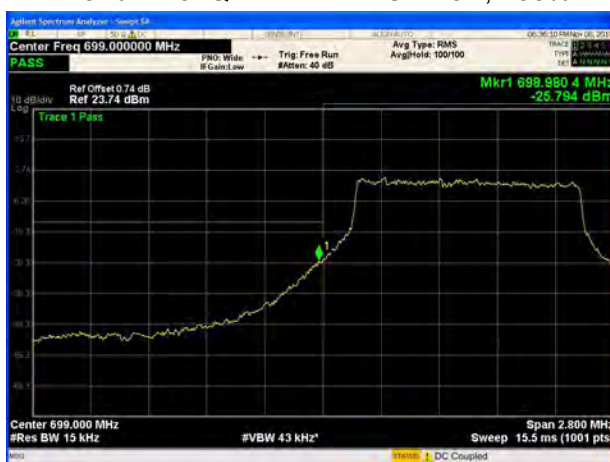
LTE Band 12 64QAM 1.4MHz CH-Low, 100%RB
