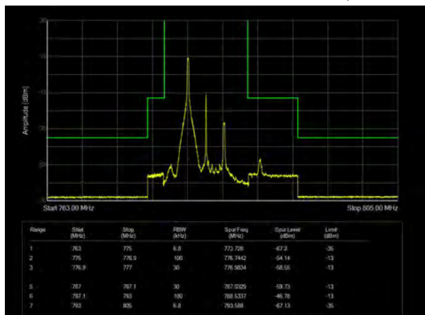
LTE Band 13 64QAM 5MHz CH-Low, 100%RB
