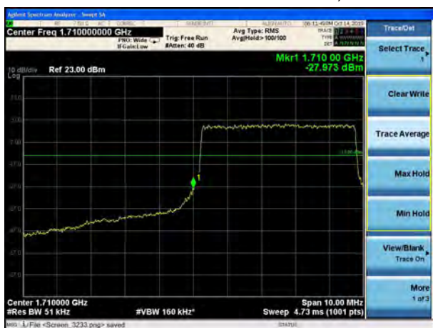
LTE Band 66 16QAM 5MHz CH-Low, 100%RB
