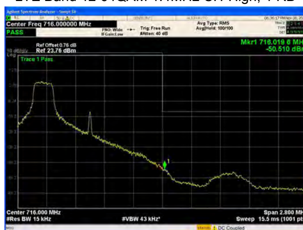
LTE Band 12 64QAM 1.4MHz CH-High, 100%RB
