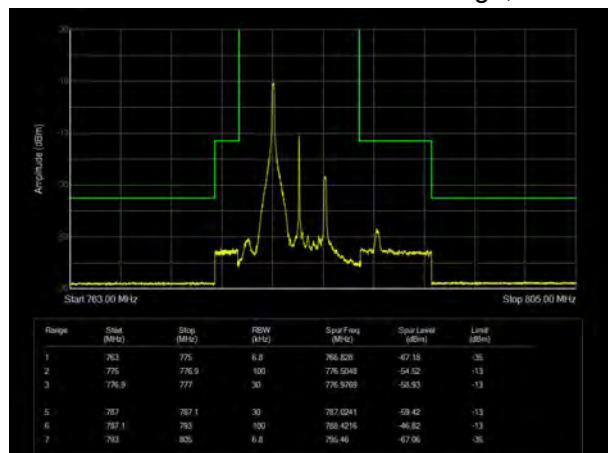
LTE Band 13 64QAM 5MHz CH-High, 100%RB
