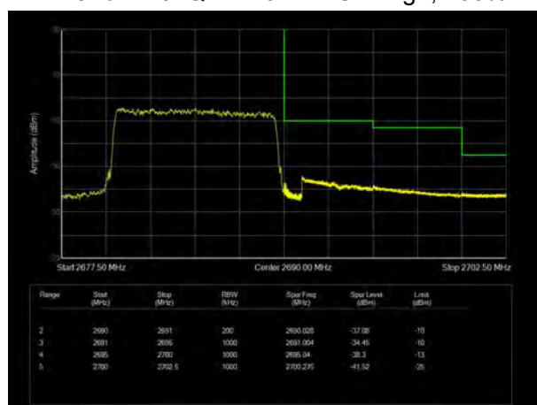
LTE Band 41 64QAM 15MHz CH-High, 1 RB
