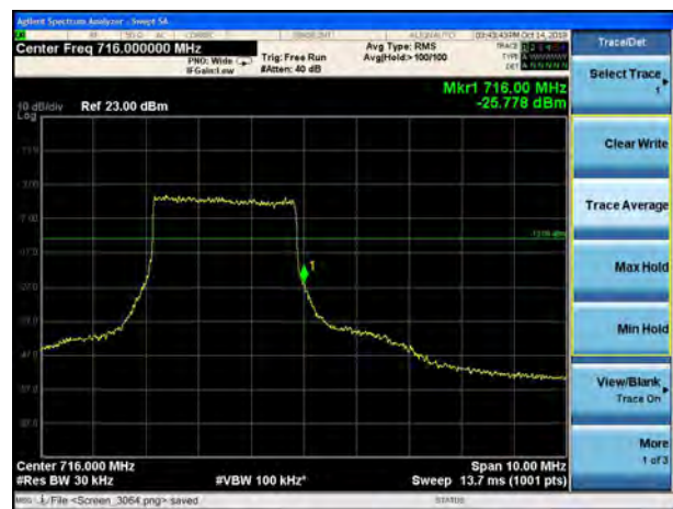
LTE Band 12 16QAM 3MHz CH-High, 100%RB
