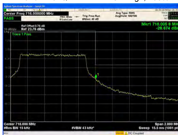
LTE Band 12 64QAM 1.4MHz CH-High, 100%RB
