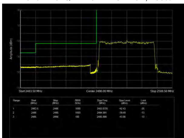
LTE Band 41 64QAM 15MHz CH-Low, 1 RB
