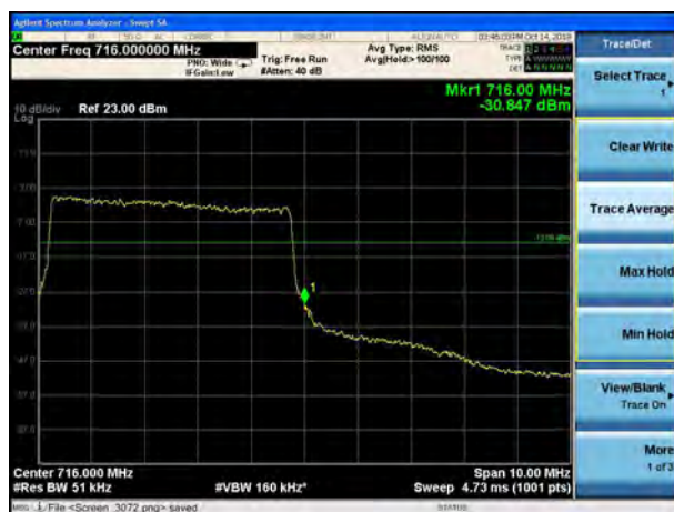
LTE Band 12 16QAM 10MHz CH-High, 1 RB
