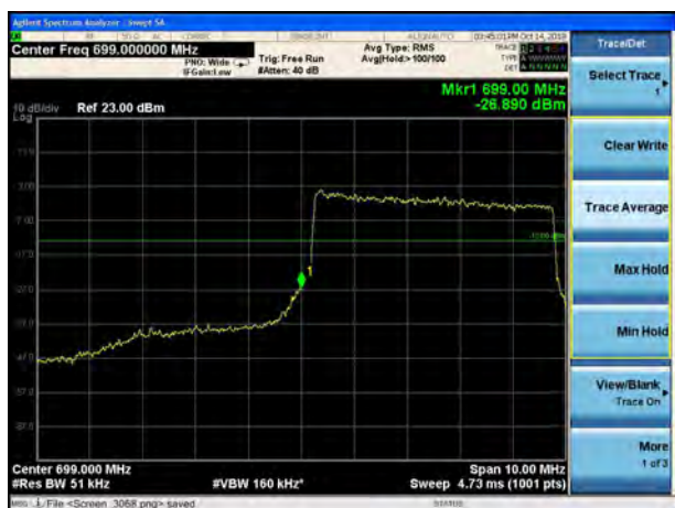
LTE Band 12 16QAM 10MHz CH-Low, 1 RB
