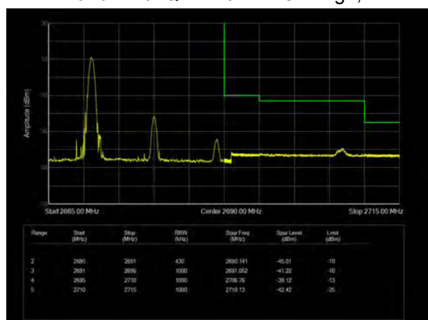
LTE Band 41 64QAM 20MHz CH-High, 100%RB
