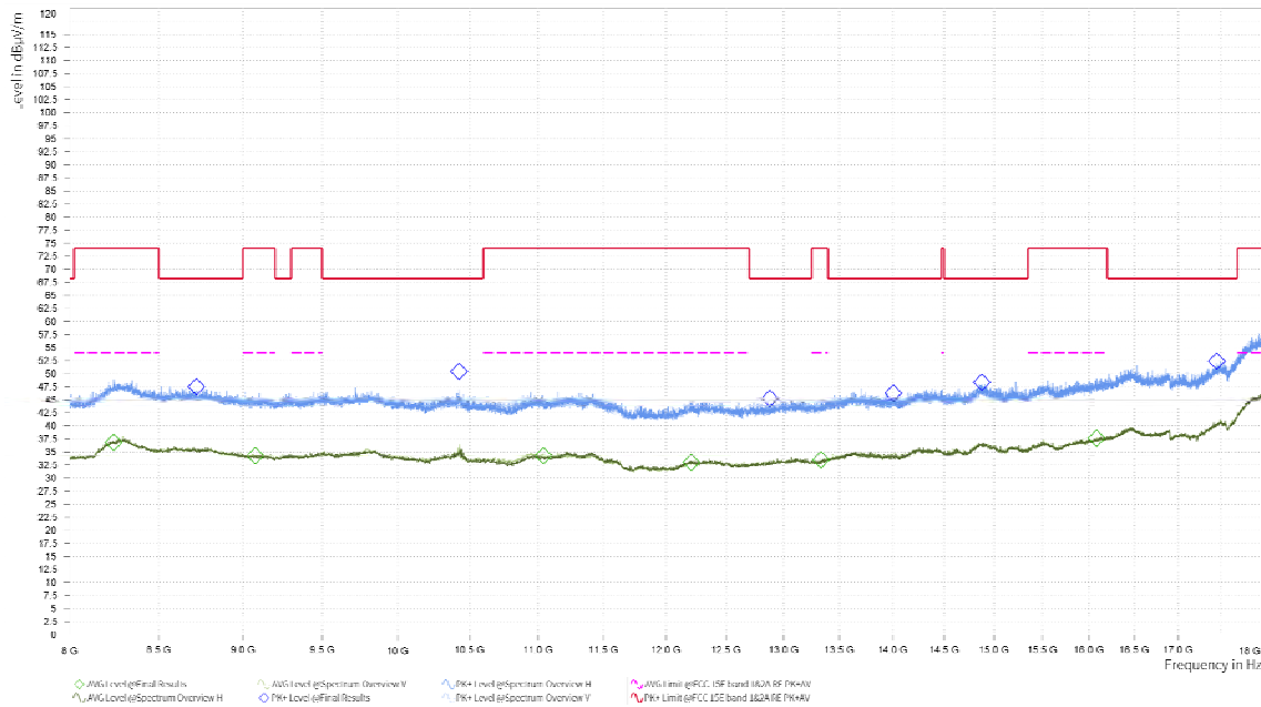
Radiates Emission from 1GHz to 8GHz
