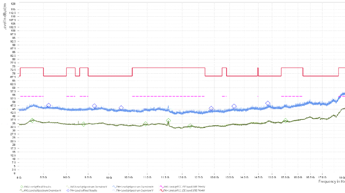
Radiates Emission from 1GHz to 8GHz
