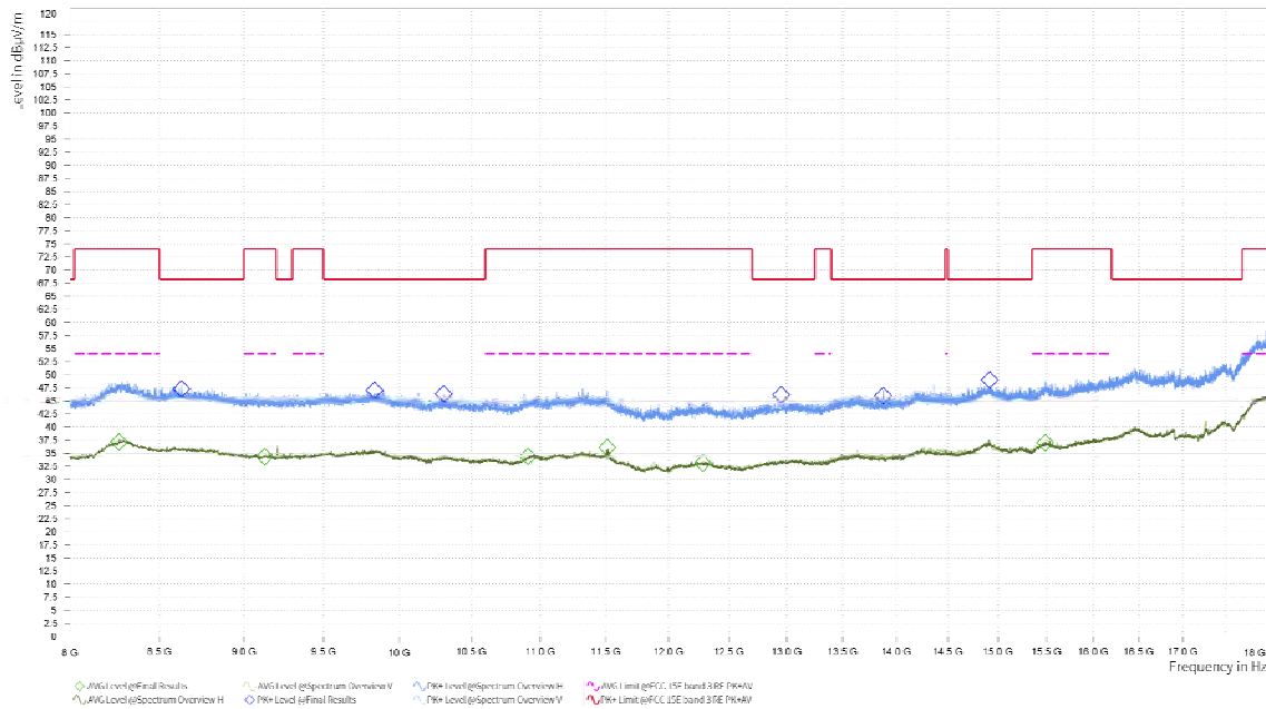
Radiates Emission from 1GHz to 8GHz
