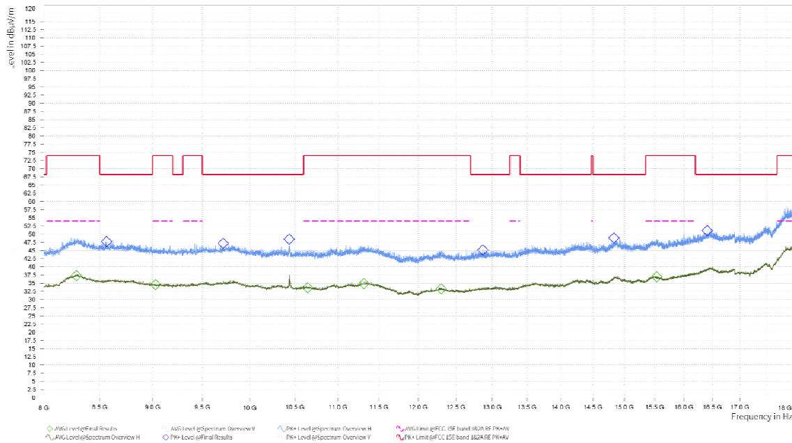
Radiates Emission from 1GHz to 8GHz
