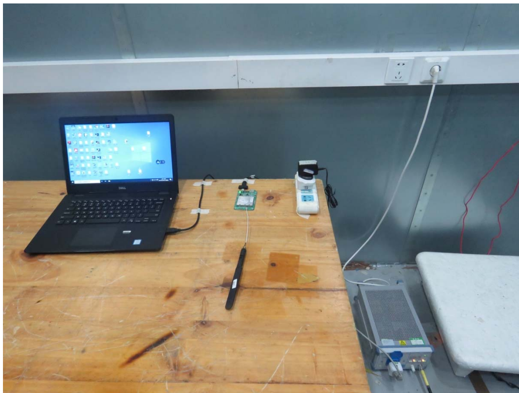
Picture 2 Conducted Emission Test Setup
