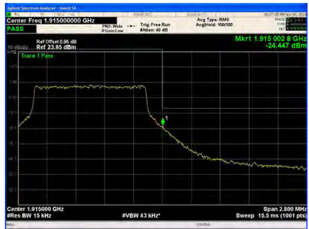
LTE Band 25 3MHz 64QAM 1RB CH-High
