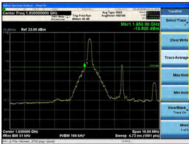
LTE Band 25 5MHz 16QAM 100%RB CH-Low
