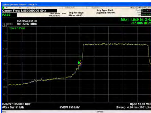
LTE Band 2 5MHz 64QAM 100%RB CH-Low
