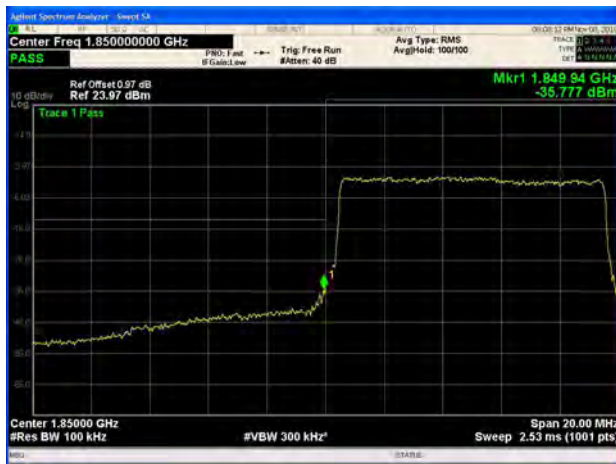
LTE Band 25 15MHz 64QAM 1RB CH-Low
