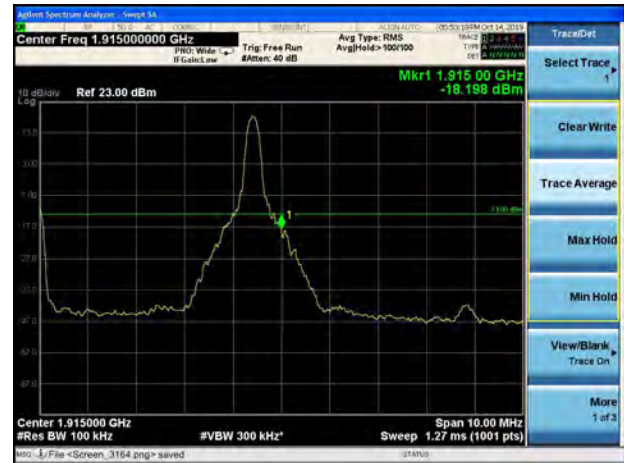
LTE Band 25 10MHz 16QAM 100%RB CH-High
