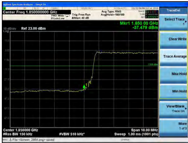
LTE Band 2 20MHz 16QAM 1RB CH-Low
