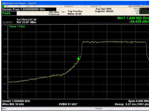
LTE Band 25 5MHz 64QAM 1RB CH-Low
