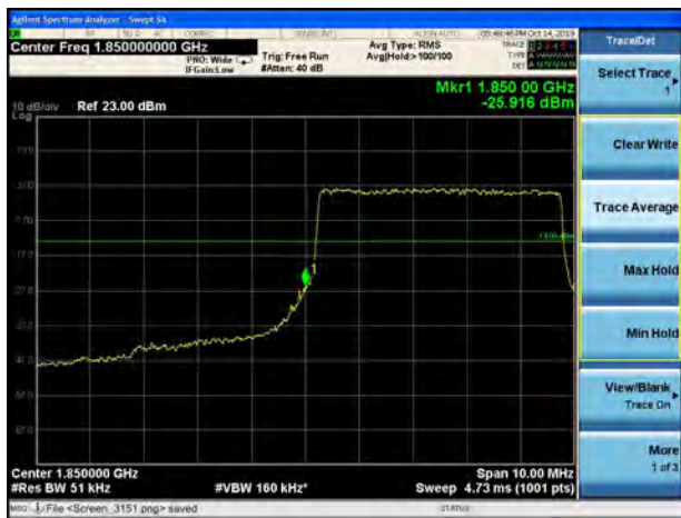
LTE Band 25 5MHz QPSK 100%RB CH-Low
