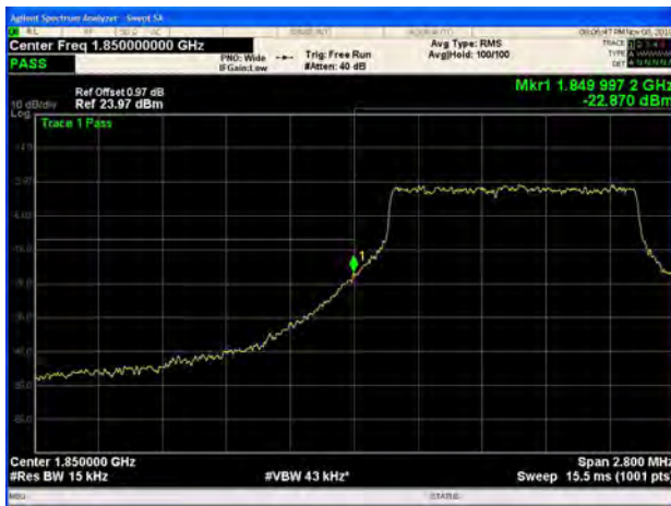
LTE Band 25 3MHz 64QAM 1RB CH-Low
