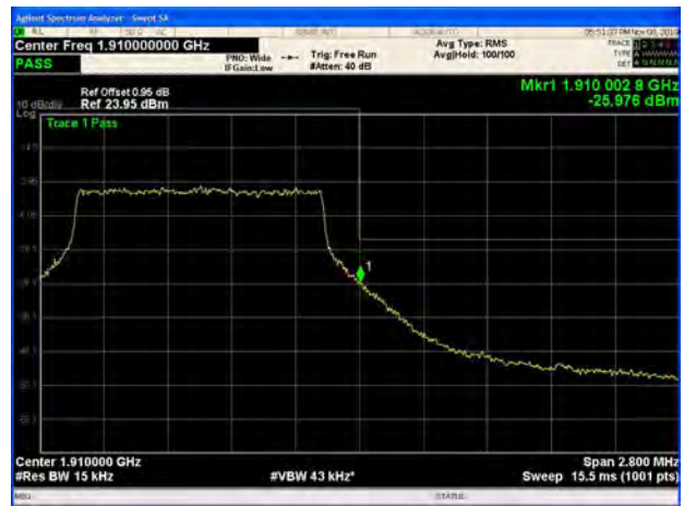
LTE Band 2 3MHz 64QAM 1RB CH-High
