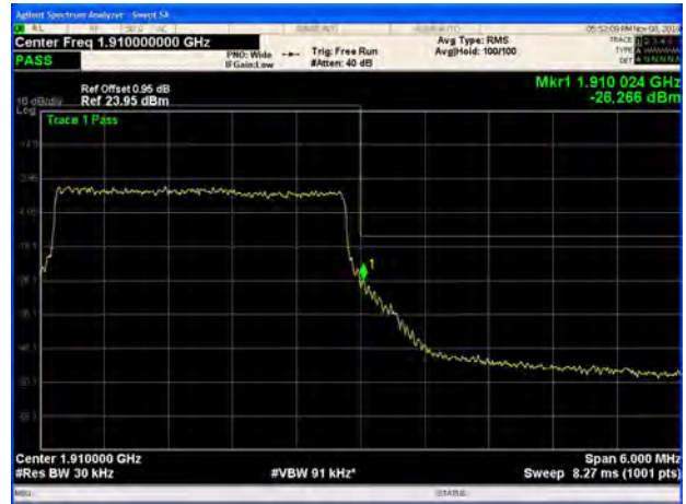
LTE Band 2 5MHz 64QAM 1RB CH-High
