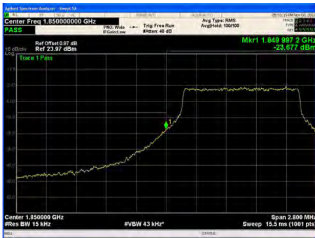
LTE Band 2 3MHz 64QAM 1RB CH-Low
