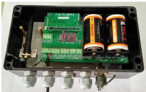
Figure 10-2: Battery replacement for Li battery option
