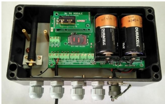
Figure 10-1: Battery replacement for Alkaline battery option
