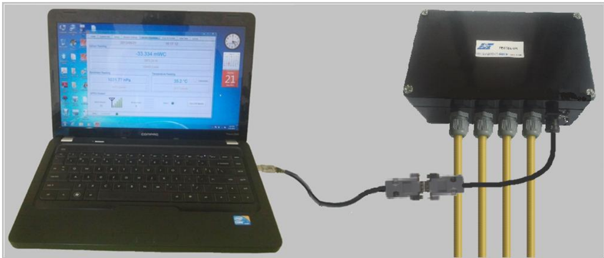
Figure 6-3: Datalogger connection using communication cable
