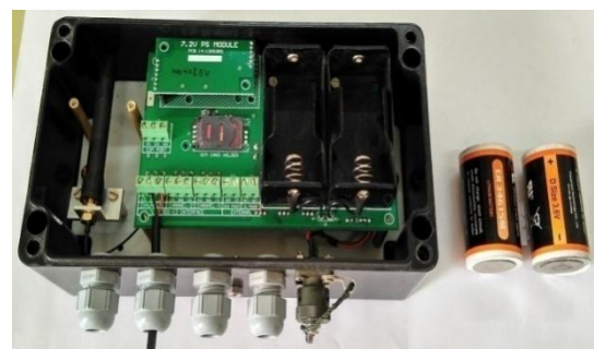
Figure 10-2: Battery replacement for Li battery option
