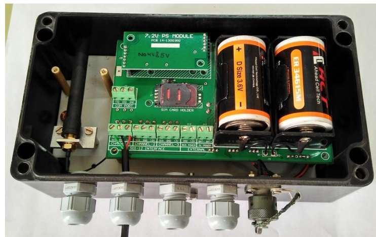
Figure 4-2 Datalogger powered with 2 x 3.6 V Lithium Batteries
