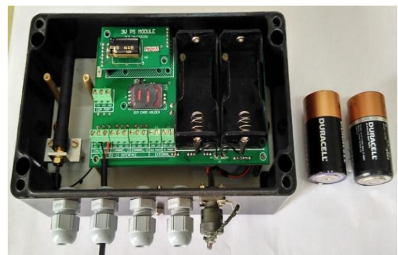
Figure 10-1: Battery replacement for Alkaline battery option
