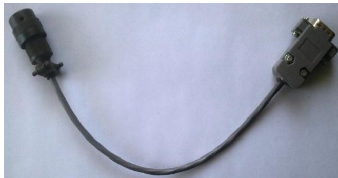
Figure 6-2: RS-232 Interface Cable
