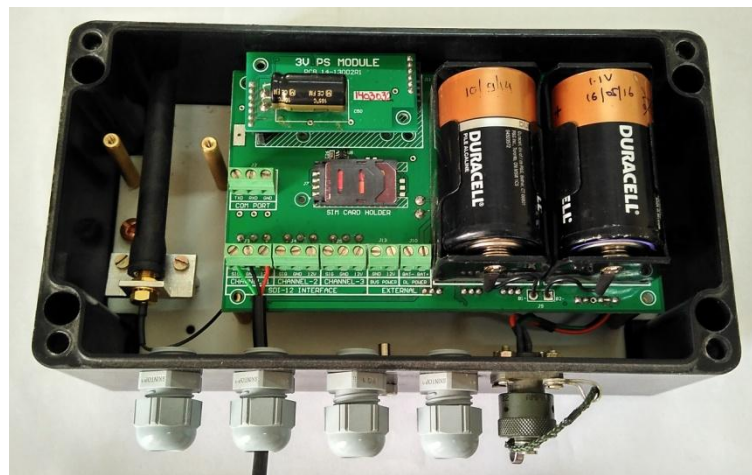
Figure 4-1 Datalogger powered with 2 x 1.5 V Alkaline Batteries
