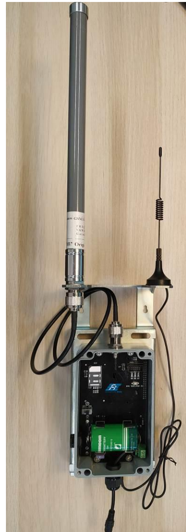
Gateway antenna & Cellular (GSM) antenna positioning
