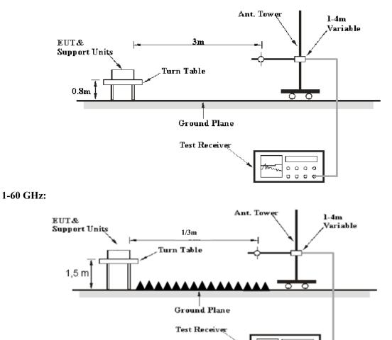
The radiated emission below 1GHz tests were performed in the 3 meters chamber test site A, above 1GHz tests were performed in the 3 meters chamber test site B, using the setup accordance with the ANSI C63.10-2013. The specification used was the FCC 15.209, and FCC 15.245 limits.
