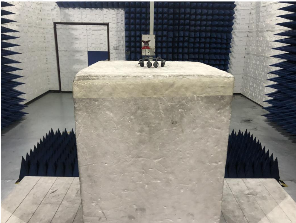
RADIATED EMISSION TEST SETUP ABOVE 1GHZ
