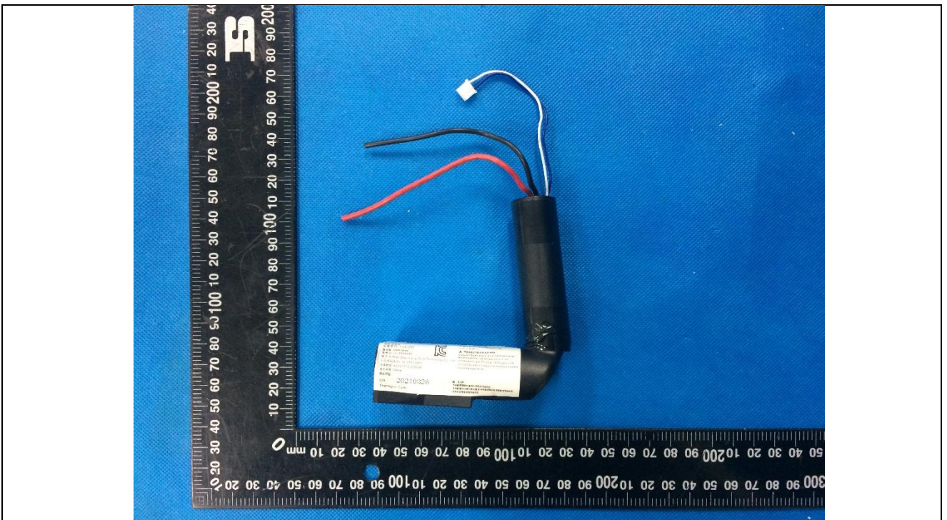
Details of: Battery pack
