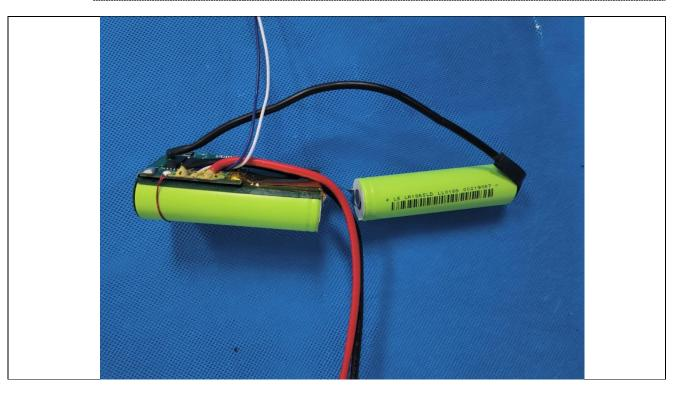
Details of: PCB view for PCM board
