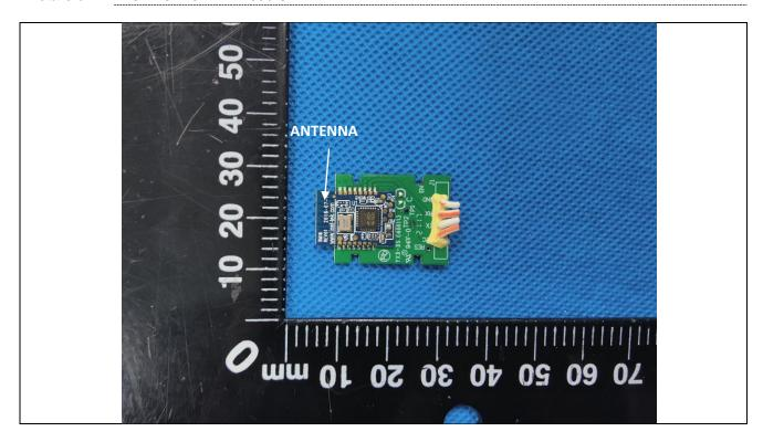
Details of: PCB view for BLE module
