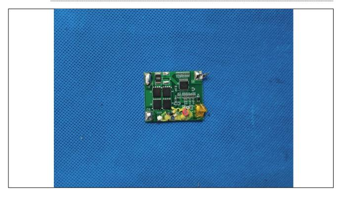
Details of: PCB view for PCM board
