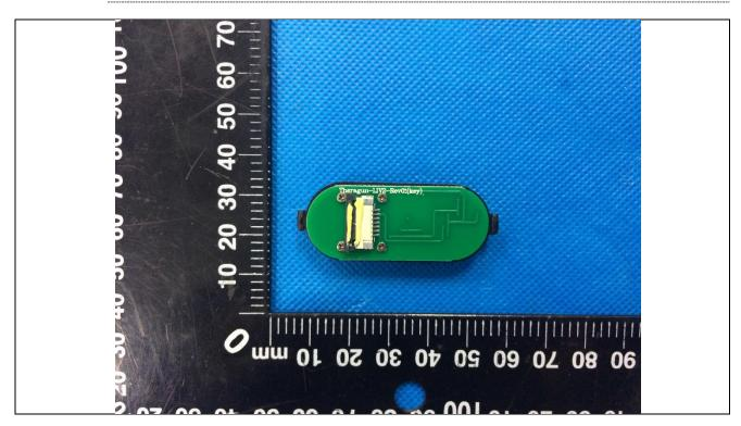
Details of: PCB view for Button board
