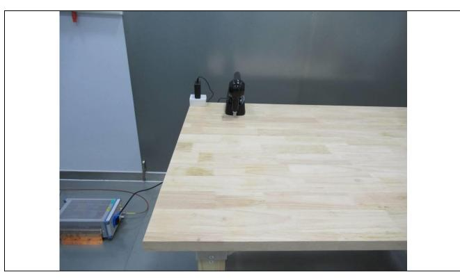
Radiated Emission test (9kHz to 30MHz)
