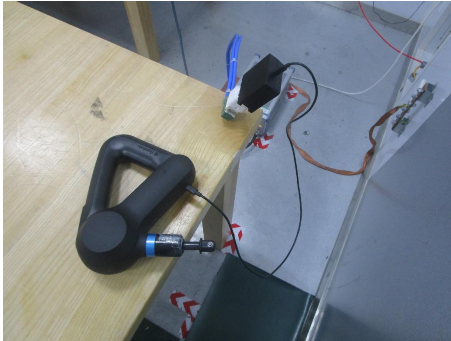
AC Power Line Conducted Emissions setup
