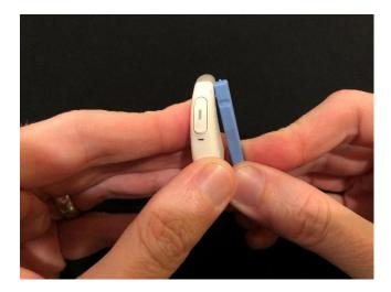
Pull the tool away from the sound processor, leaving the pin inside the sound processor.
