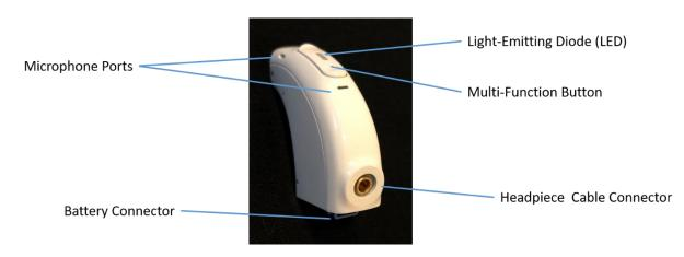
The Naída CI M90 sound processor features direct connectivity to wireless accessories and Bluetoothenabled devices. The Naída CI M90 offers multiple power options and wearing options for the user.
