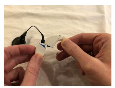
Align the battery connector with the sound processor housing side of the connector.
