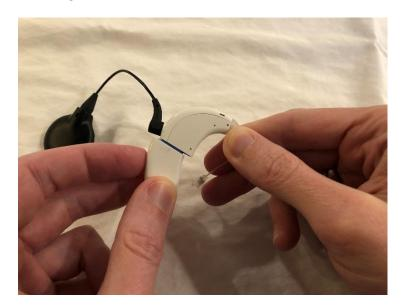
Slide the battery onto the sound processor until it clicks into place. Do not force the battery onto the sound processor. The batteries are designed to be inserted in only one direction; applying force may damage the equipment.
