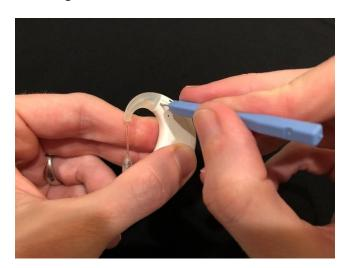
Gently press the tool in the hole, pushing the pin out the other side.
