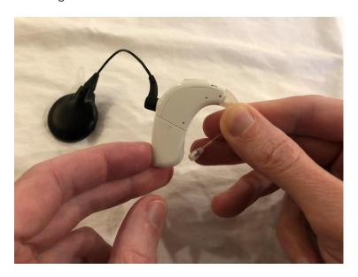
Firmly slide the battery away from the M T-Mic, M Earhook, or M Acoustic Earhook.
