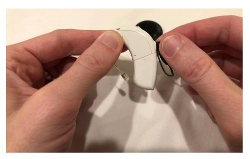
NOTE: To maximize cable life, the cable should only be unplugged from the sound processor when changing wearing configuration or when replacing the cable.
