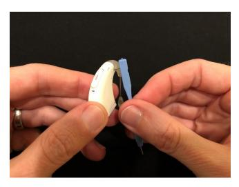
If a small portion of the pin extends beyond the sound processor, use the side of the tool to push the pin inwards so it lies flush with the sound processor.
