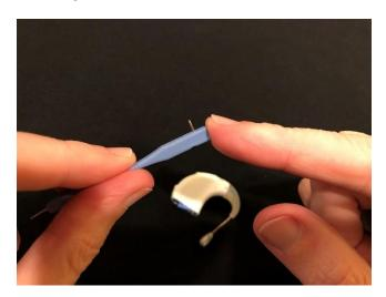
Line up the pin with the hole in the earhook and gently push it through the hole. The pin will move from one side of the sound processor, through the earhook to the other side of the sound processor, holding the earhook in place. The pin should not come out the other side.
