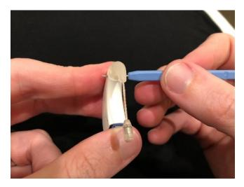
The pin does not need to be removed from the sound processor. As long as the tool is pushed in flush on one side of the sound processor, the pin should be displaced enough to adequately remove the earhook. Remove the tool from the sound processor. Gently grasp the earhook at the top near where it connects with the sound processor and pull forward until it is separated from the sound processor.
