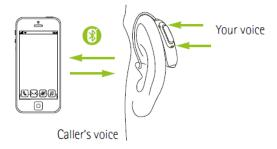
When making a phone call, you will hear a dialing tone through the sound processor. The sound processor microphones pick up your voice. When receiving a call, a call notification will be heard through the sound processor. You can accept the call with a short press on the upper or lower part of the multifunction button on the sound processor or directly on the phone.
