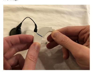
Continue sliding the battery until it separates from the sound processor.
