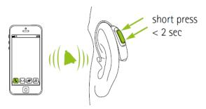
You can reject or end a call with a long press on the upper or lower part of the multifunction button on the sound processor or directly through the phone.
