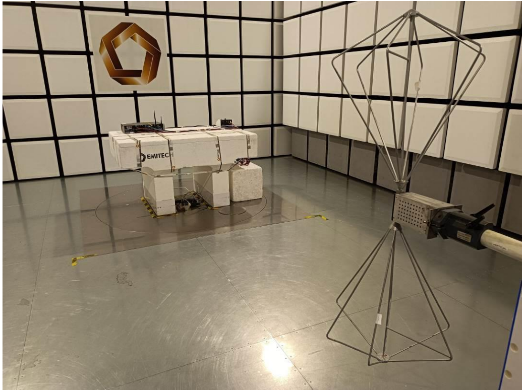
TEST SETUP PHOTO(S) – SETUP FOR FREQ < 200MHZ
