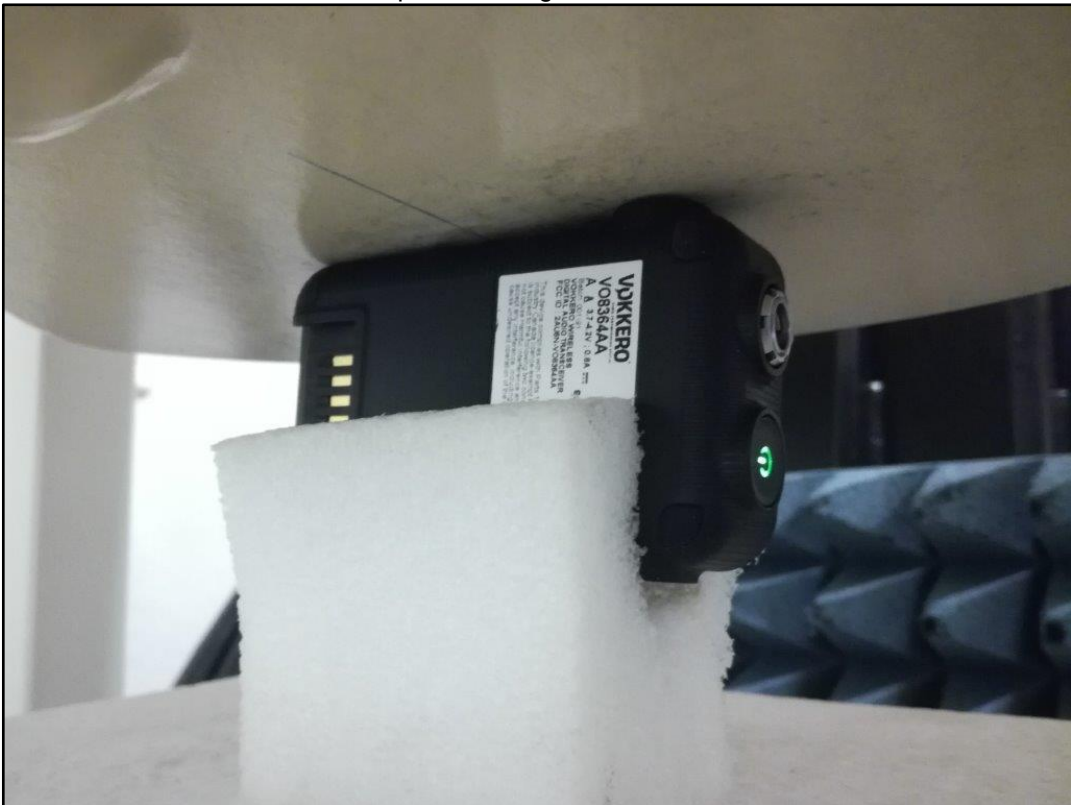
Photo 10: Test position - Right side with 0mm distance
