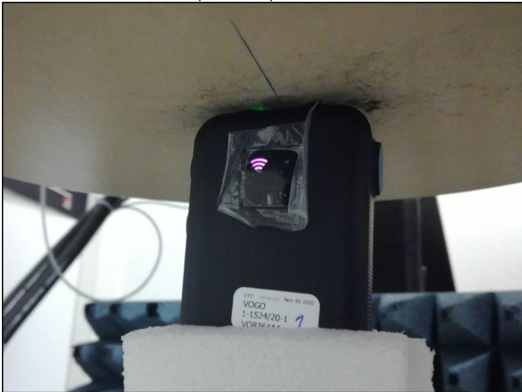
Photo 12: Test position - Bottom side with 0mm distance
