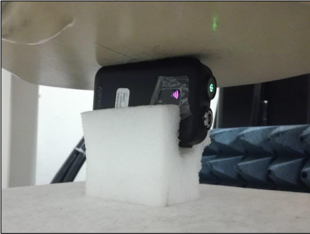
Photo 10: Test position - Right side with 0mm distance
