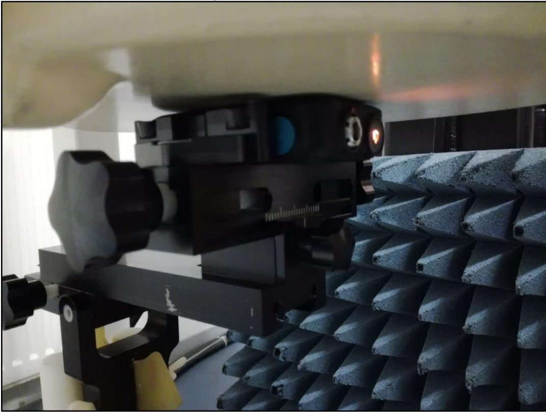
Photo 8: Test position - Rear with 0mm distance
