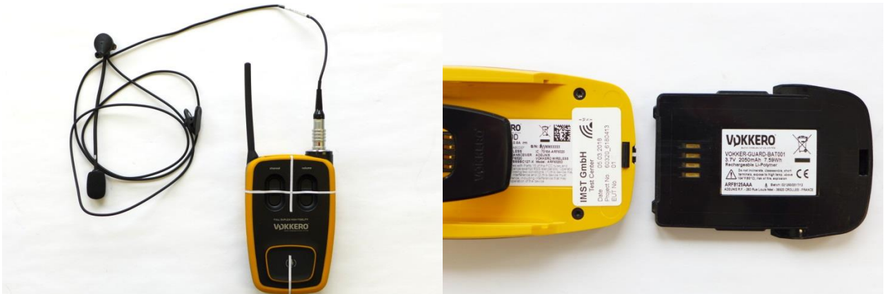
Pic. 3: Device under test with attached headset and detached battery.
