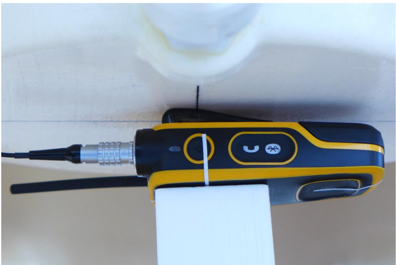
Pic. 4: Test position back side of EUT towards the phantom with attached belt clip and headset.
