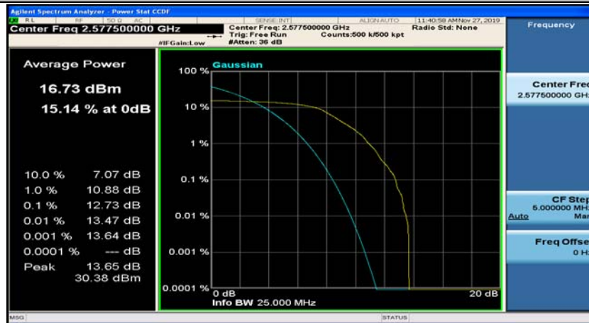
(Channel Bandwidth:15 MHz)_LCH_QPSK_1RB#37
