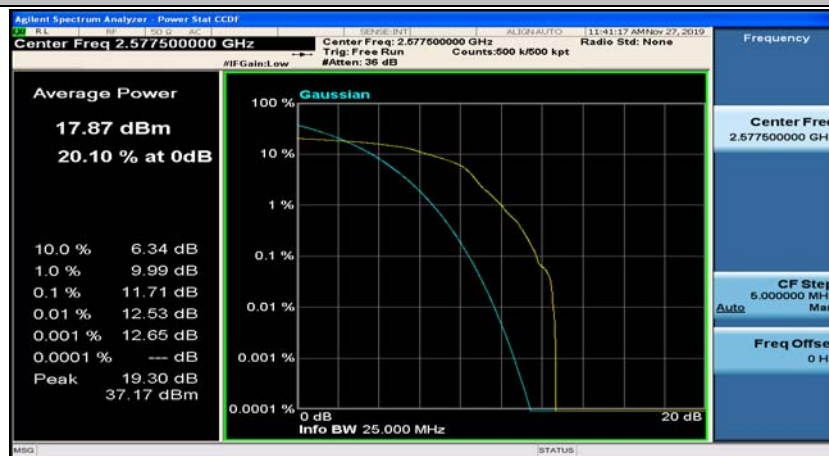
(Channel Bandwidth:15 MHz)_LCH_16QAM_1RB#37
