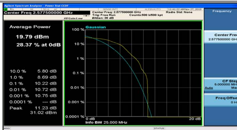
(Channel Bandwidth:15 MHz)_LCH_16QAM_1RB#74
