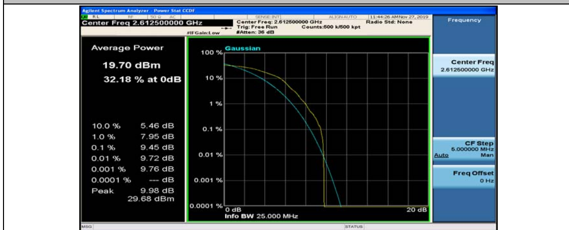
(Channel Bandwidth:15 MHz)_HCH_16QAM_1RB#37
