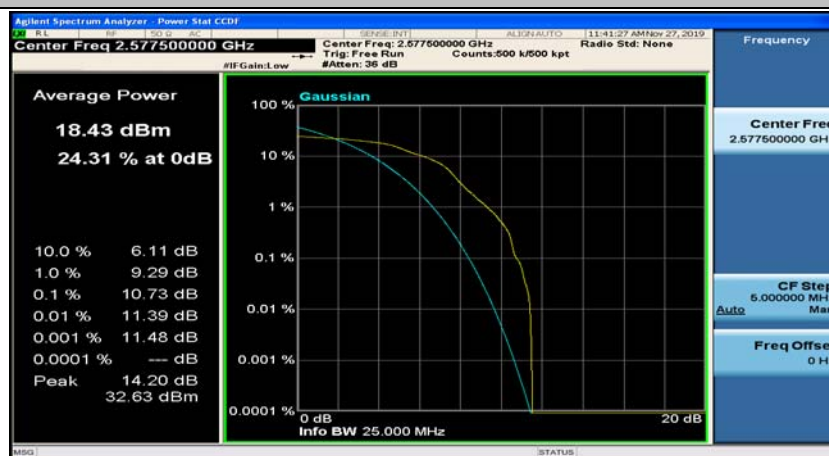
(Channel Bandwidth:15 MHz)_LCH_16QAM_37RB#0
