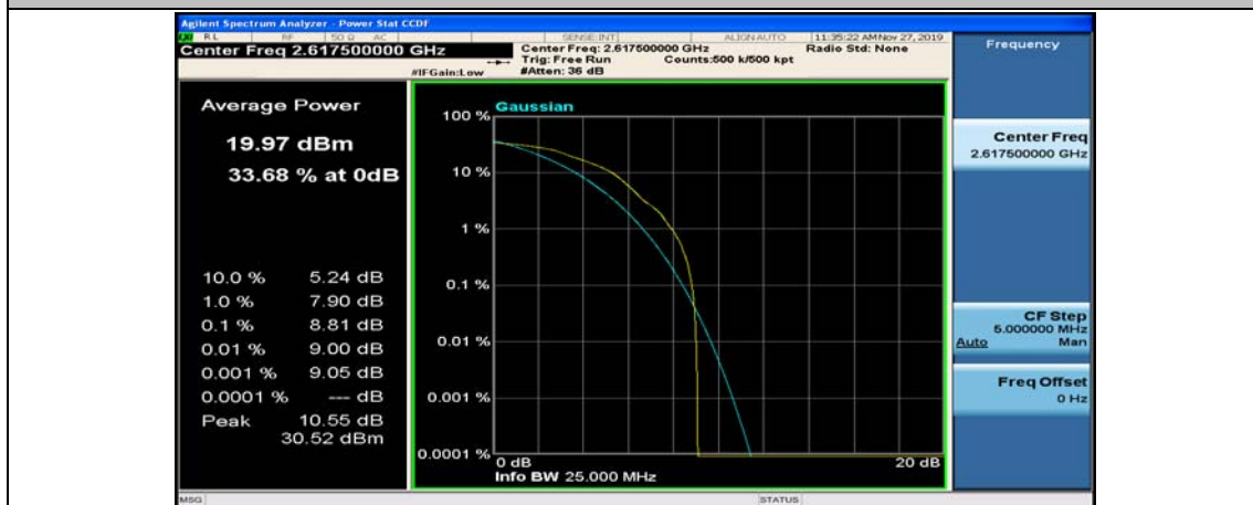
(Channel Bandwidth: 5 MHz)_HCH_16QAM_1RB#12
