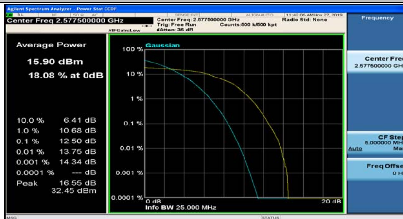
(Channel Bandwidth:15 MHz)_LCH_16QAM_75RB#0
