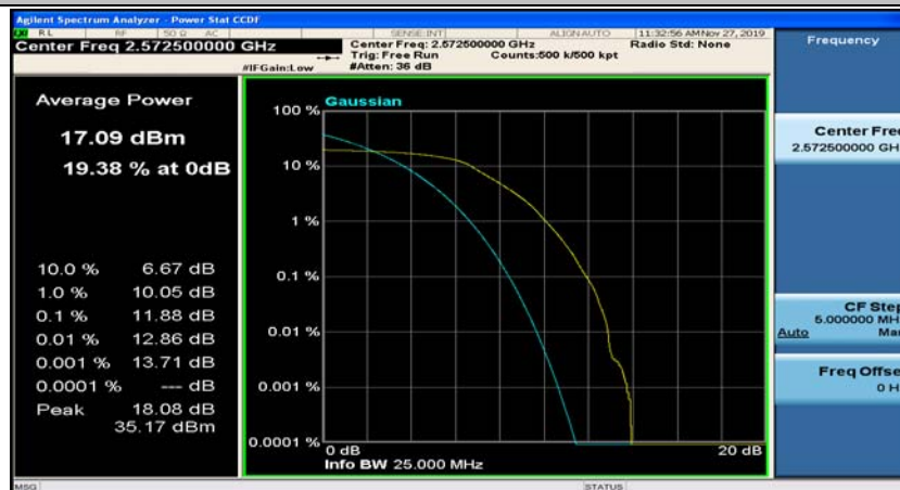
(Channel Bandwidth: 5 MHz)_LCH_QPSK_25RB#0
