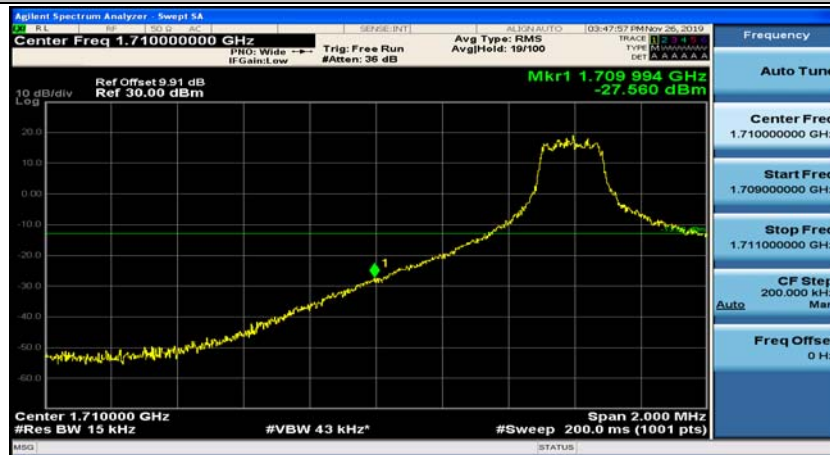
Channel Bandwidth: 10 MHz_LCH_QPSK_1RB#24
