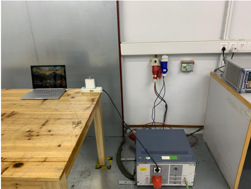
RADIATED EMISSION TEST SETUP BELOW 1GHZ
