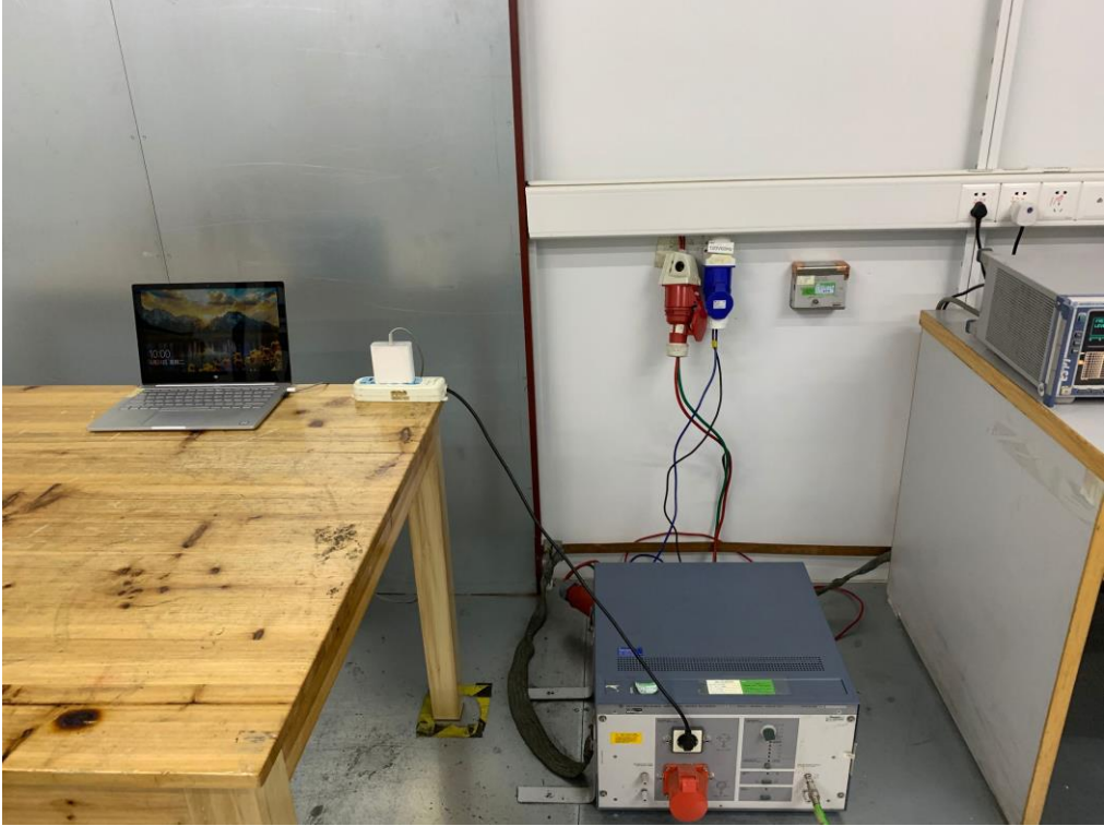
RADIATED EMISSION TEST SETUP BELOW 1GHZ
